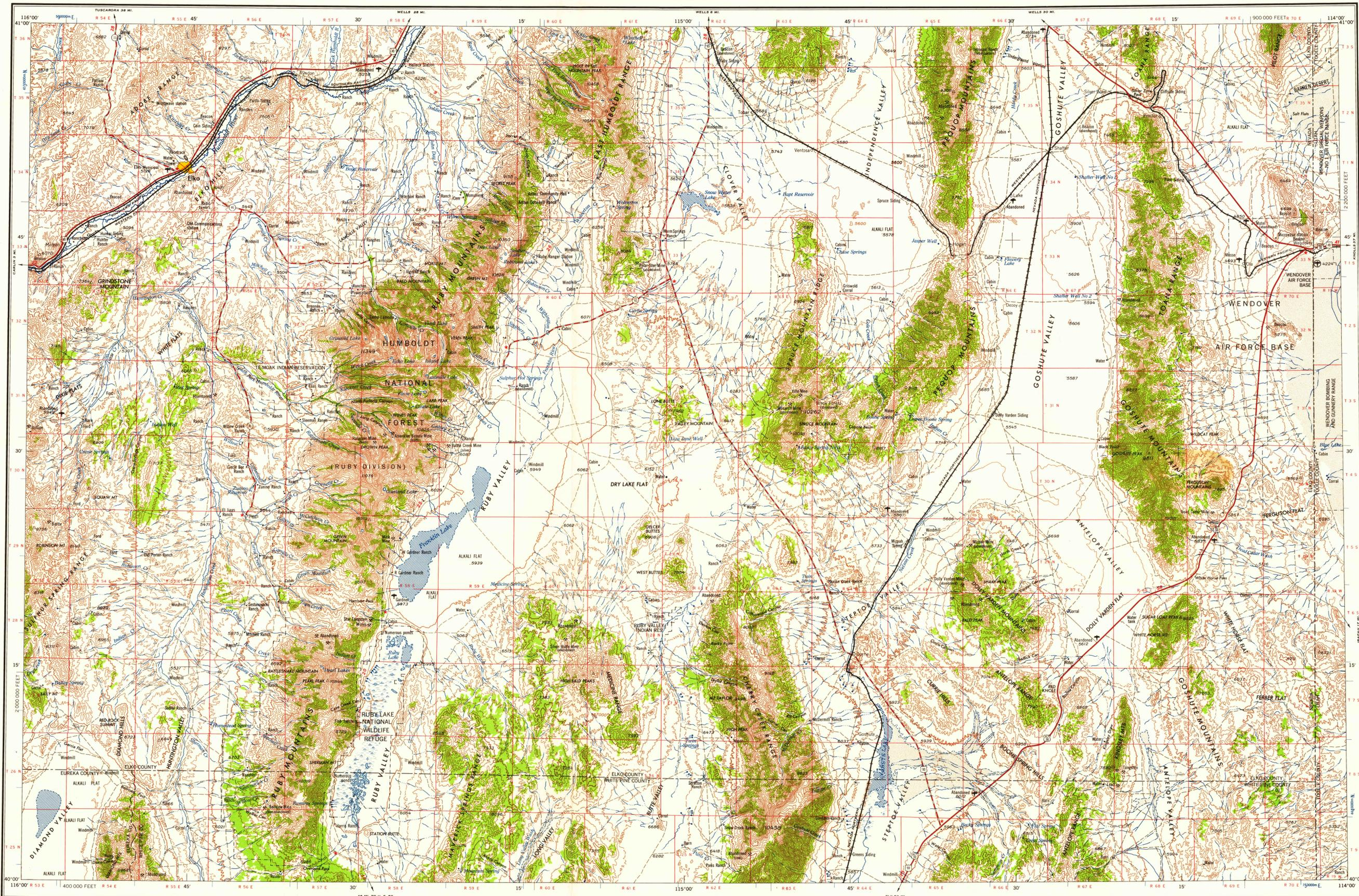
Prepared by the Army Map Service (KCSK), Corps of Engineers, U. S. Army, Washington, D. C. Compiled in 1956 by photogrammetric methods. Horizontal and vertical control by USGS, USGS and CE. Aerial photography 1953-54. Photography field annotated 1955. 100,000-foot grid based on Nevada coordinate system, east zone 10,000-meter Universal Transverse Mercator grid ticks, zone 11, shown in blue.
