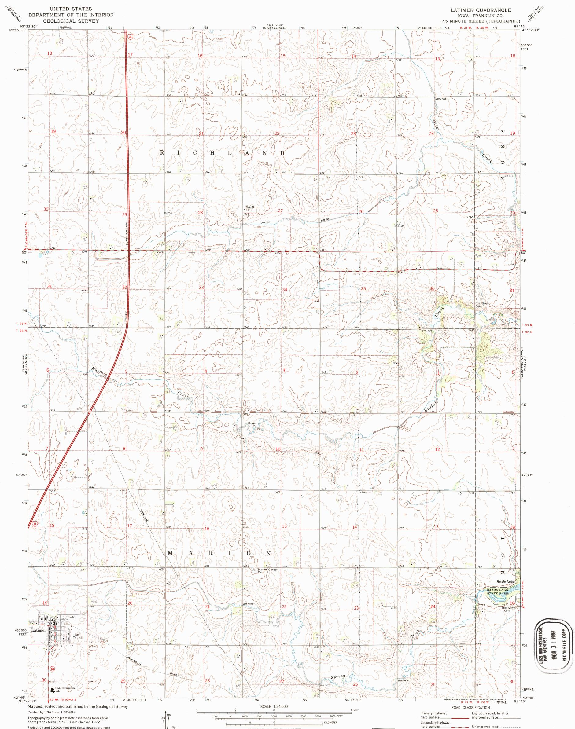
Projection and 10,000-foot grid ticks: Iowa coordinate system, north zone (Lambert conformal conic) 1000-meter Universal Transverse Mercator grid ticks, zone 15, shown in blue. 1927 North American datum Fine red dashed lines indicate selected fence and field lines where
