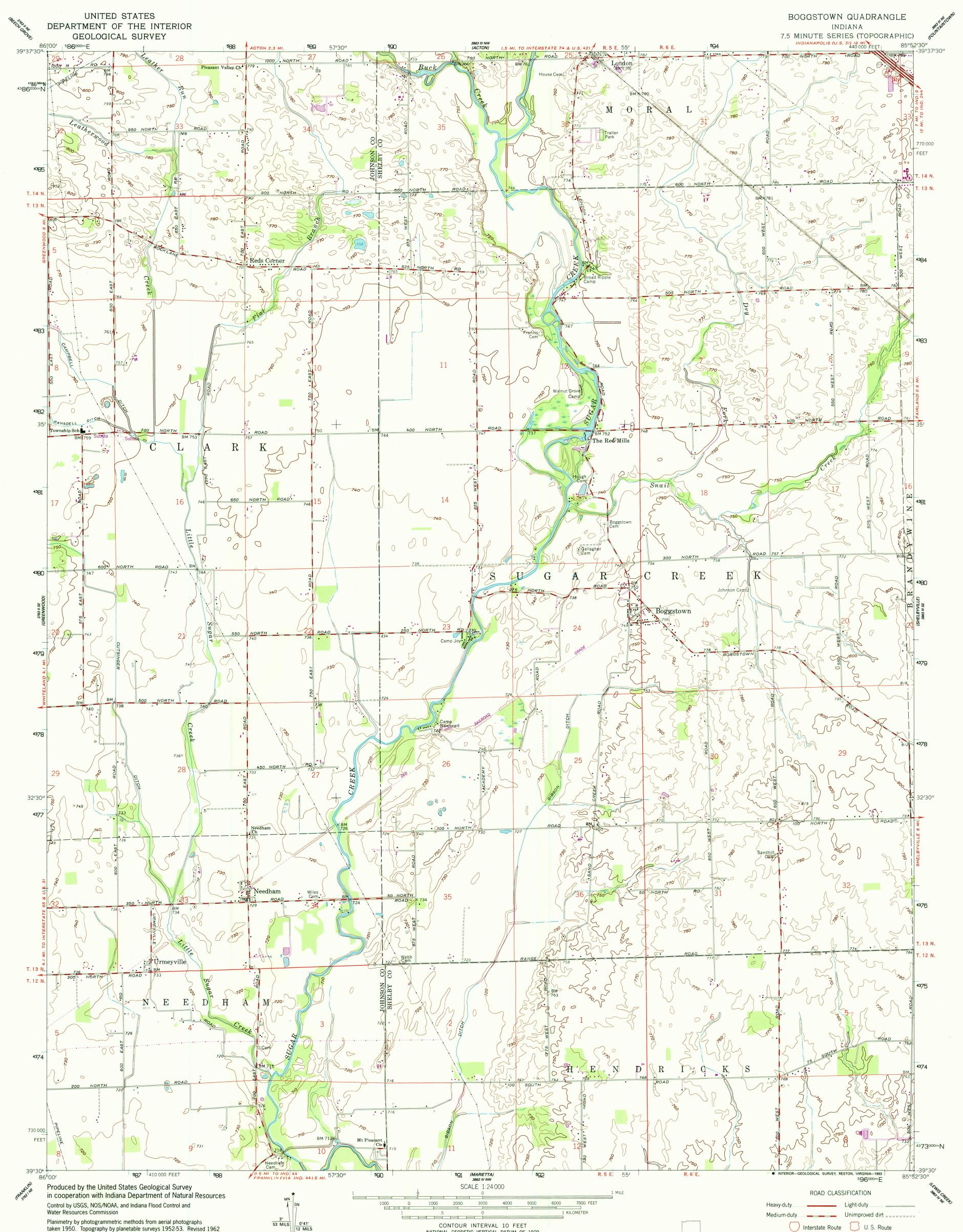
Planimetry by photogrammetric methods from aerial photographs taken 1950. Topography by planetable surveys 1952-53. Revised 1962
