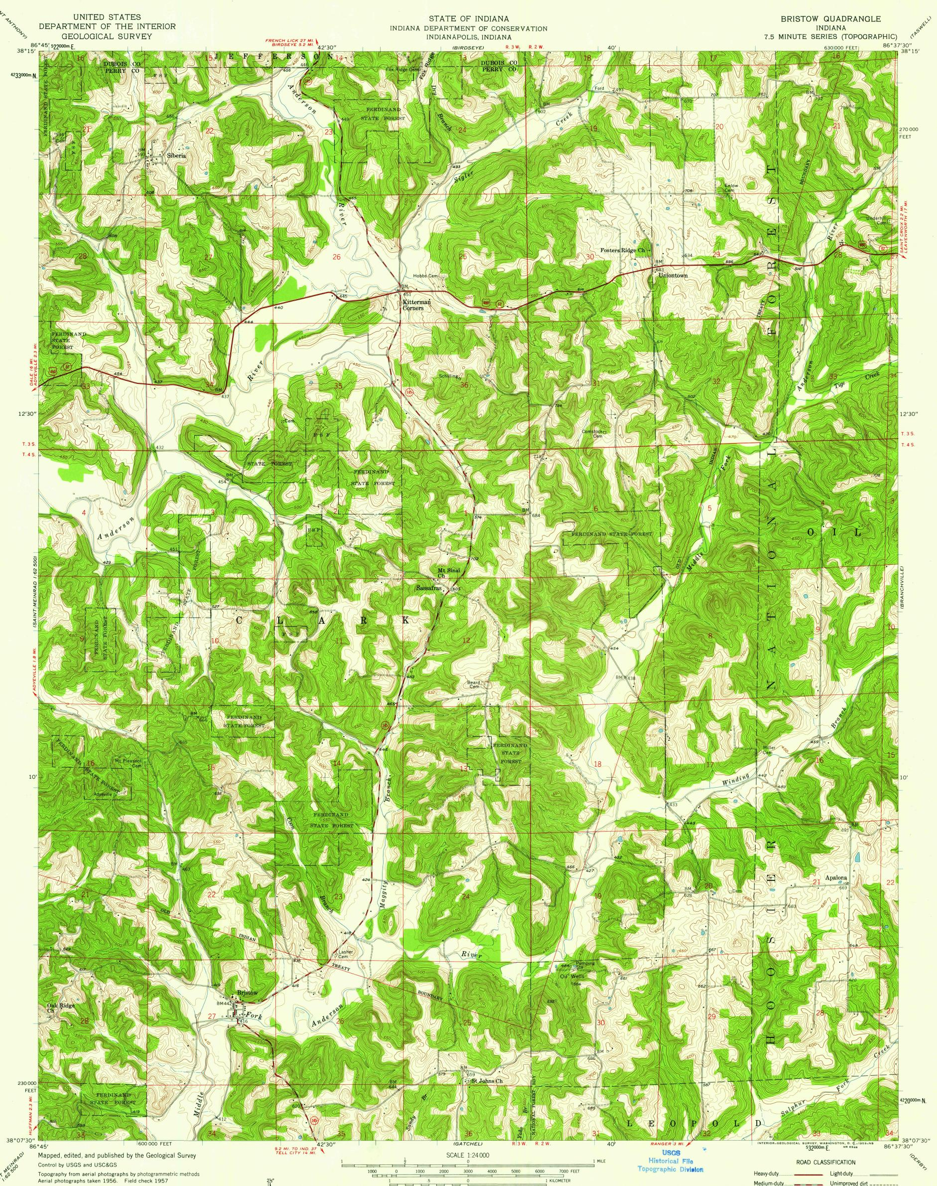
Polyconic projection. 1927 North American datum 10,000-foot grid based on Indiana coordinate system, west zone 1000-meter Universal Transverse Mercator grid ticks, zone 16, shown in blue Unchecked elevations are shown in brown
