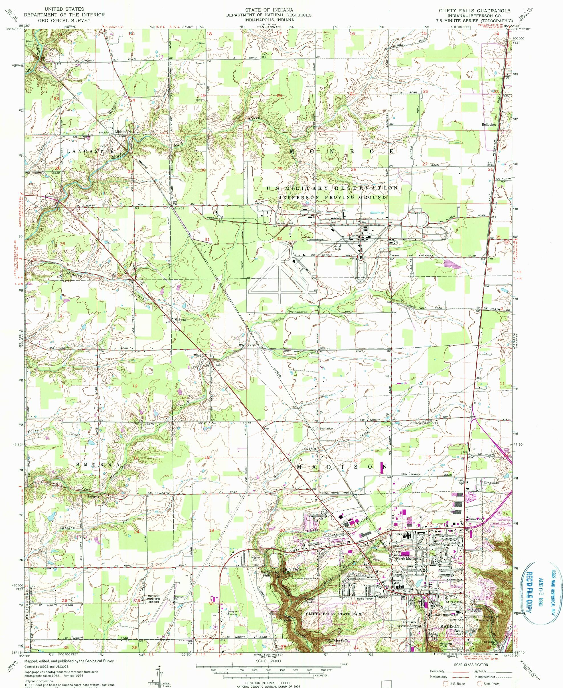
10,000-foot grid based on Indiana coordinate system, east zone 1000-meter Universal Transverse Mercator grid ticks, zone 16. shown in blue. 1927 North American Datum To place on the predicted North American Datum 1983 move the projection lines 3 meters south and 3 meters west as shown by dashed corner ticks
