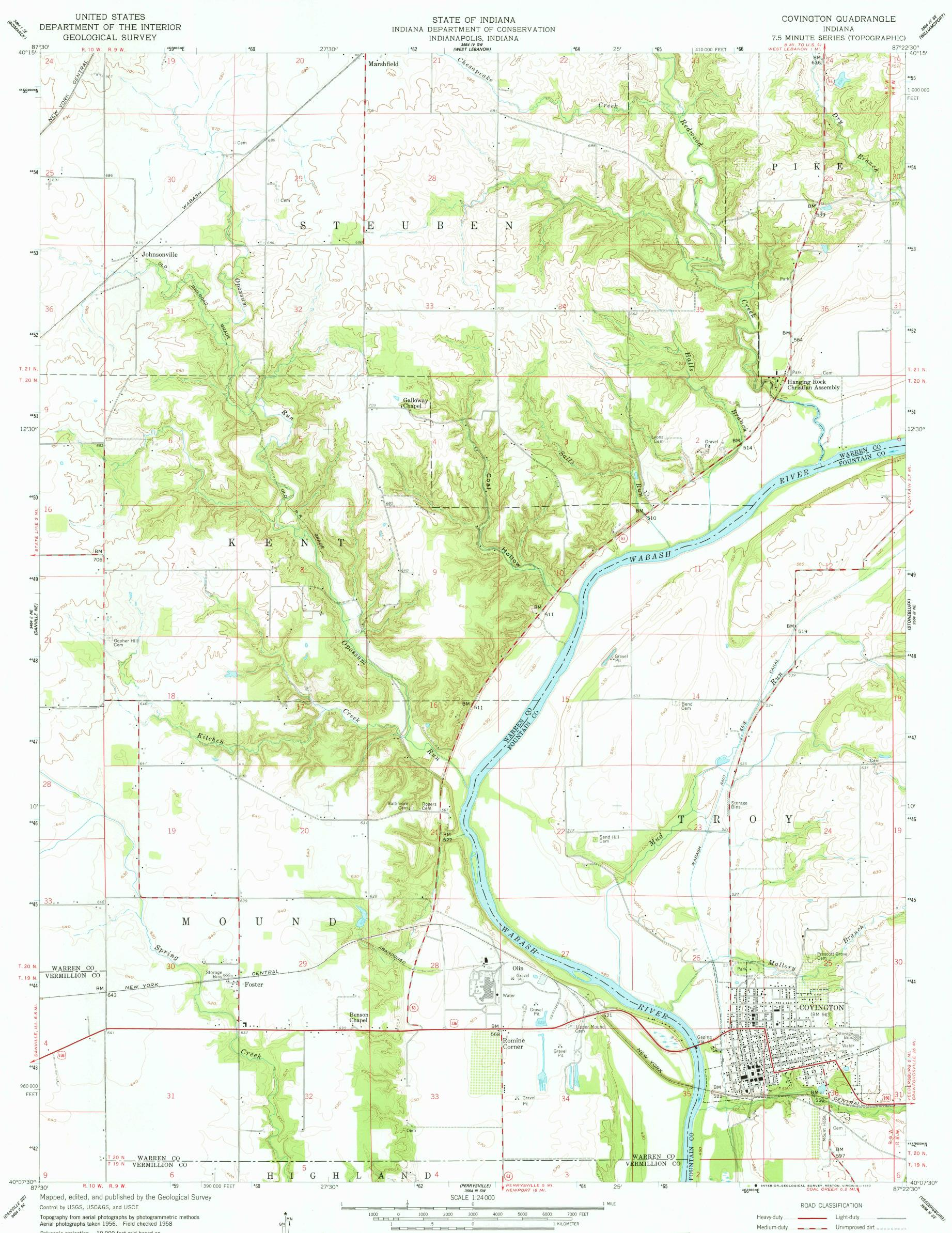
Polyconic projection. 10,000-foot grid based on Indiana coordinate system, west zone 1000-meter Universal Transverse Mercator grid ticks, zone 16, shown in blue. 1927 North American Datum To place on the predicted North American Datum 1983 move the projection lines 3 meters east as shown by dashed corner ticks Unchecked elevations are shown in brown
