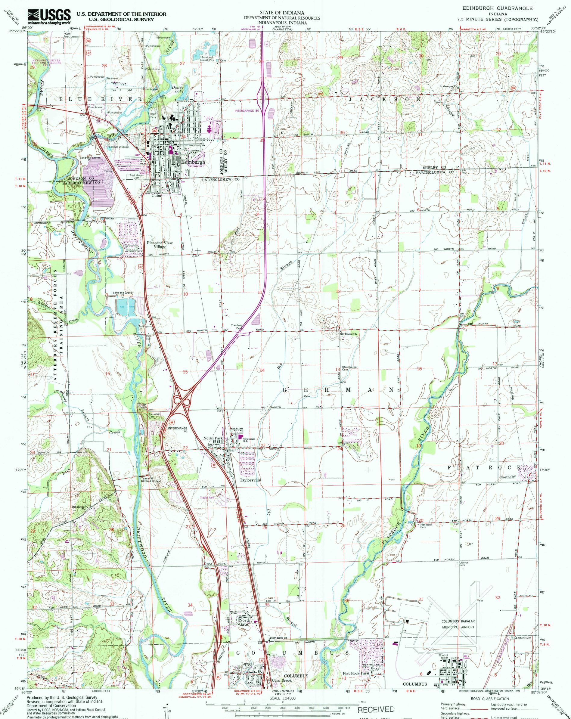
Planimetry by photogrammetric methods from aerial photographs taken 1944. Topography by planetable surveys 1946-47. Revised 1961 Projection and 10,000-foot grid ticks: Indiana coordinate system, east zone (transverse Mercator) 1000-meter Universal Transverse Mercator grid ticks, zone 16, shown in blue 1927 North American Datum of 1982 (NAD 82) is chown by dechad ecome ticks
