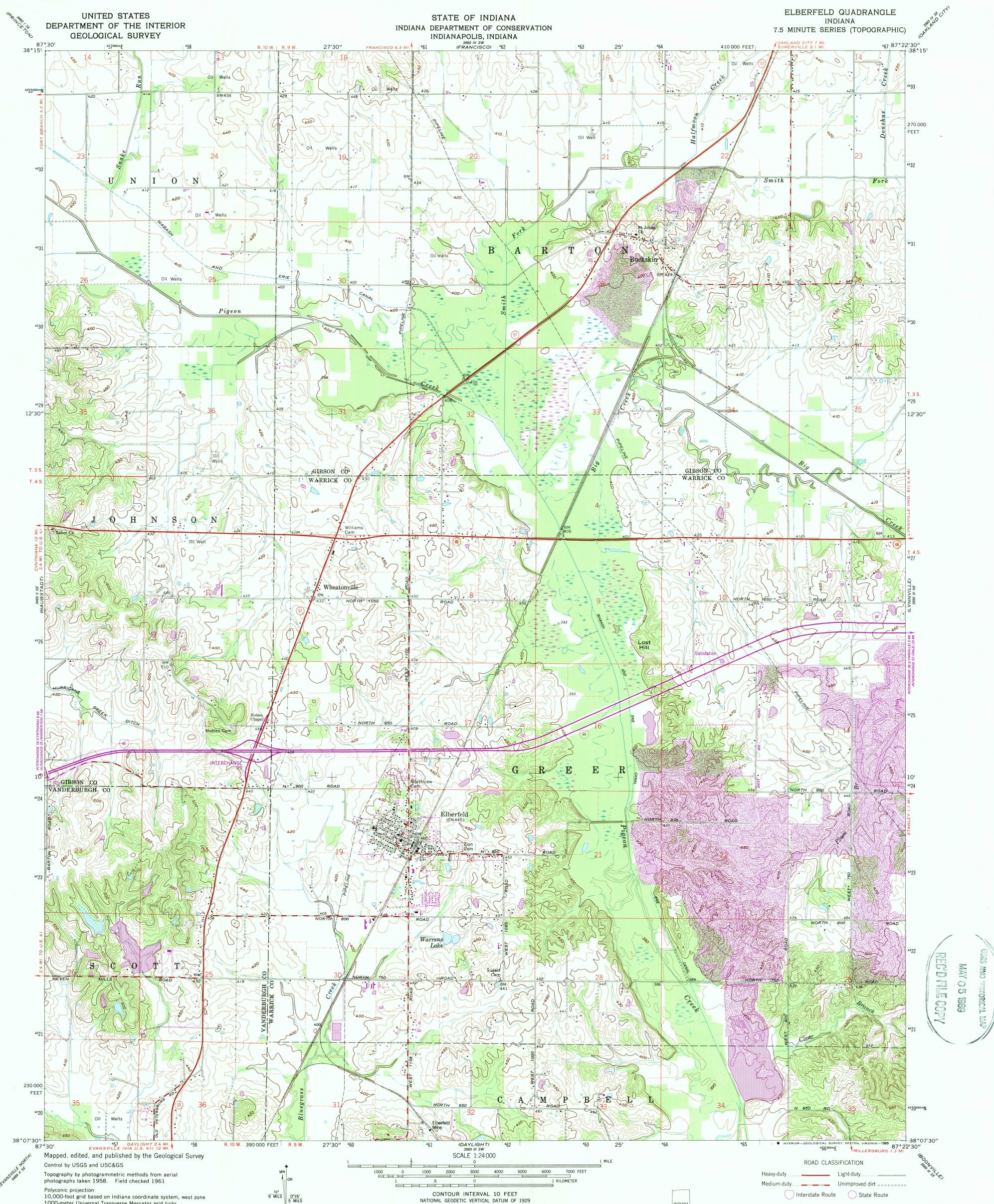
10,000-foot grid based on Indiana coordinate system, west zone 1000-meter Universal Transverse Mercator grid ticks, zone 16, shown in blue. 1927 North American Datum To place on the predicted North American Datum 1983 move the projection lines 3 meters south and 2 meters east as shown by dashed corner ticks
