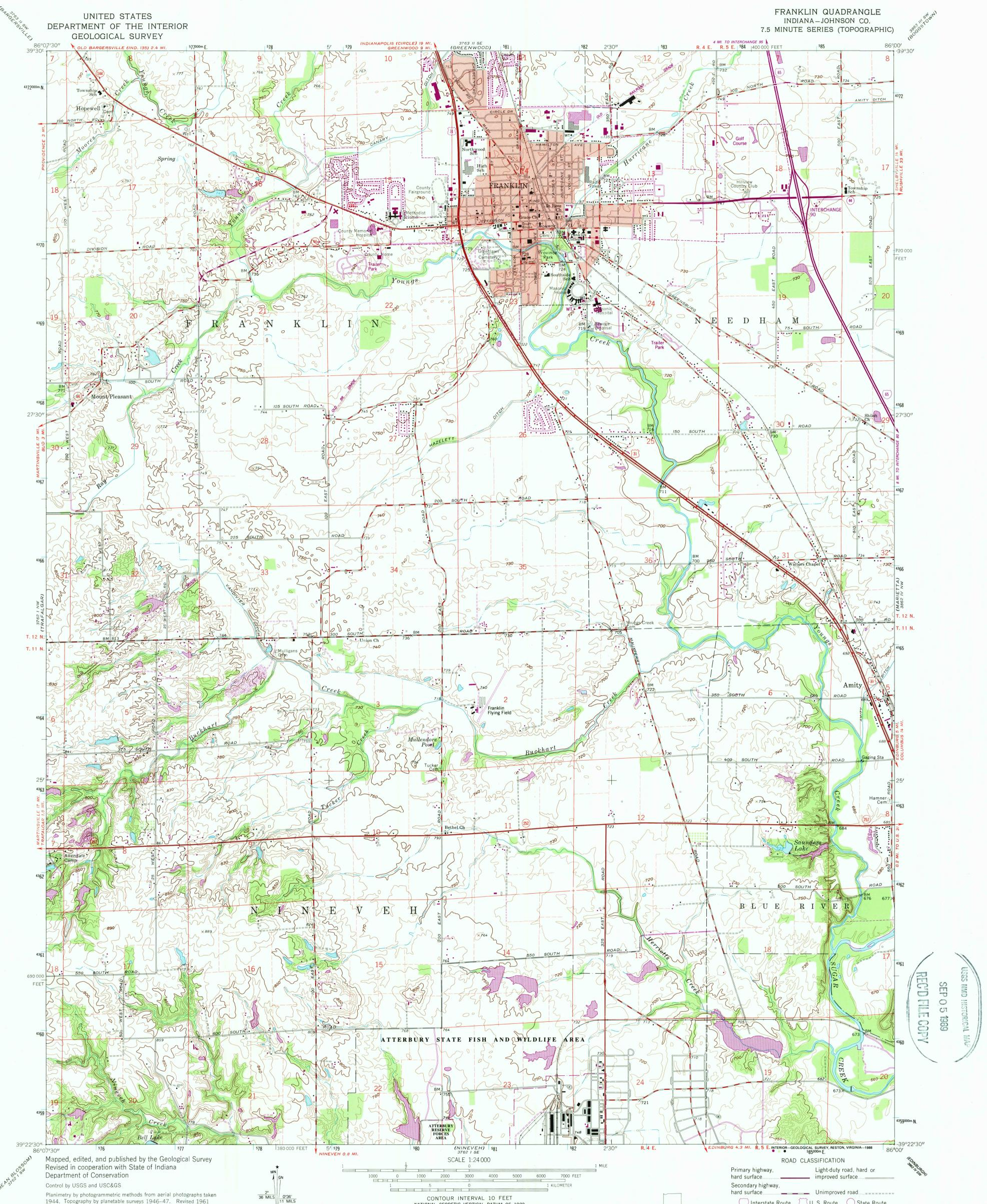
Planimetry by photogrammetric methods from aerial photographs taken 1944. Topography by planetable surveys 1946-47. Revised 1961
