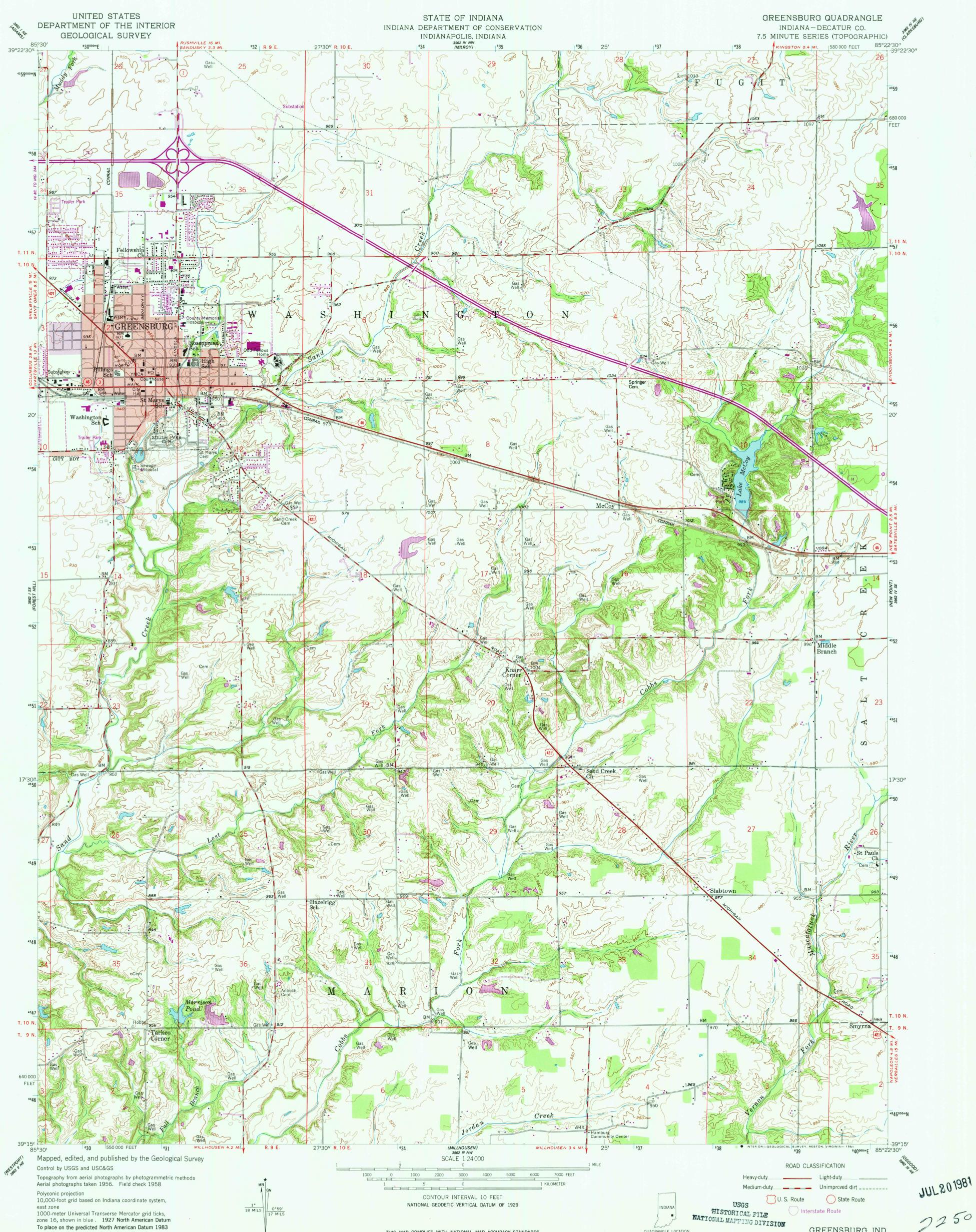
Polyconic projection 10,000-foot grid based on Indiana coordinate system, east zone 1000-meter Universal Transverse Mercator grid ticks, zone 16, shown in blue . 1927 North American Datum To place on the predicted North American Datum 1983 move the projection lines 2 meters south and 3 meters west as shown by dashed corner ticks
