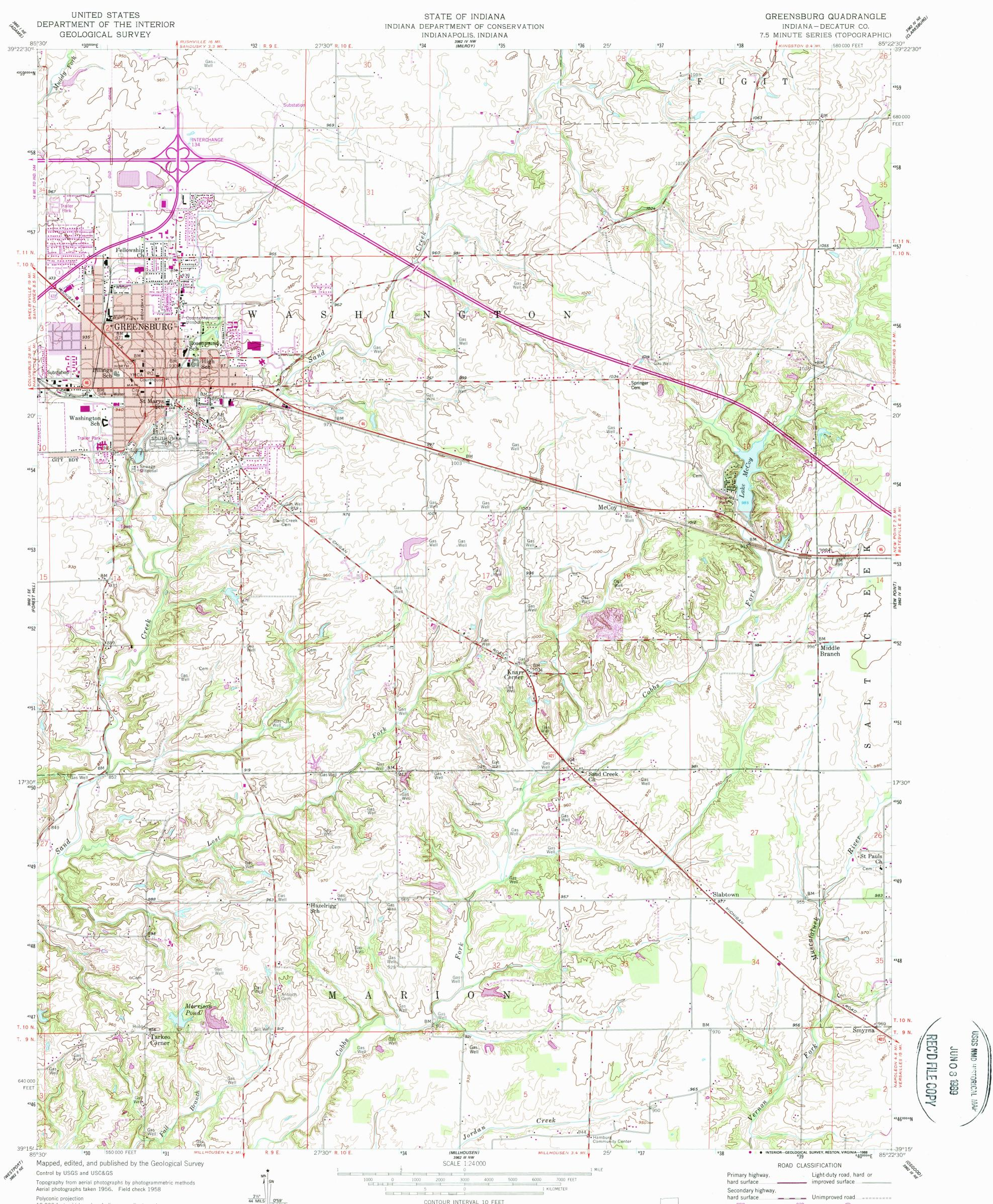
Polyconic projection 10,000-foot grid based on Indiana coordinate system, east zone 1000-meter Universal Transverse Mercator grid ticks, zone 16, shown in blue . 1927 North American Datum To place on the predicted North American Datum 1983 move the projection lines 2 meters south and 3 meters west as shown by dashed corner ticks
