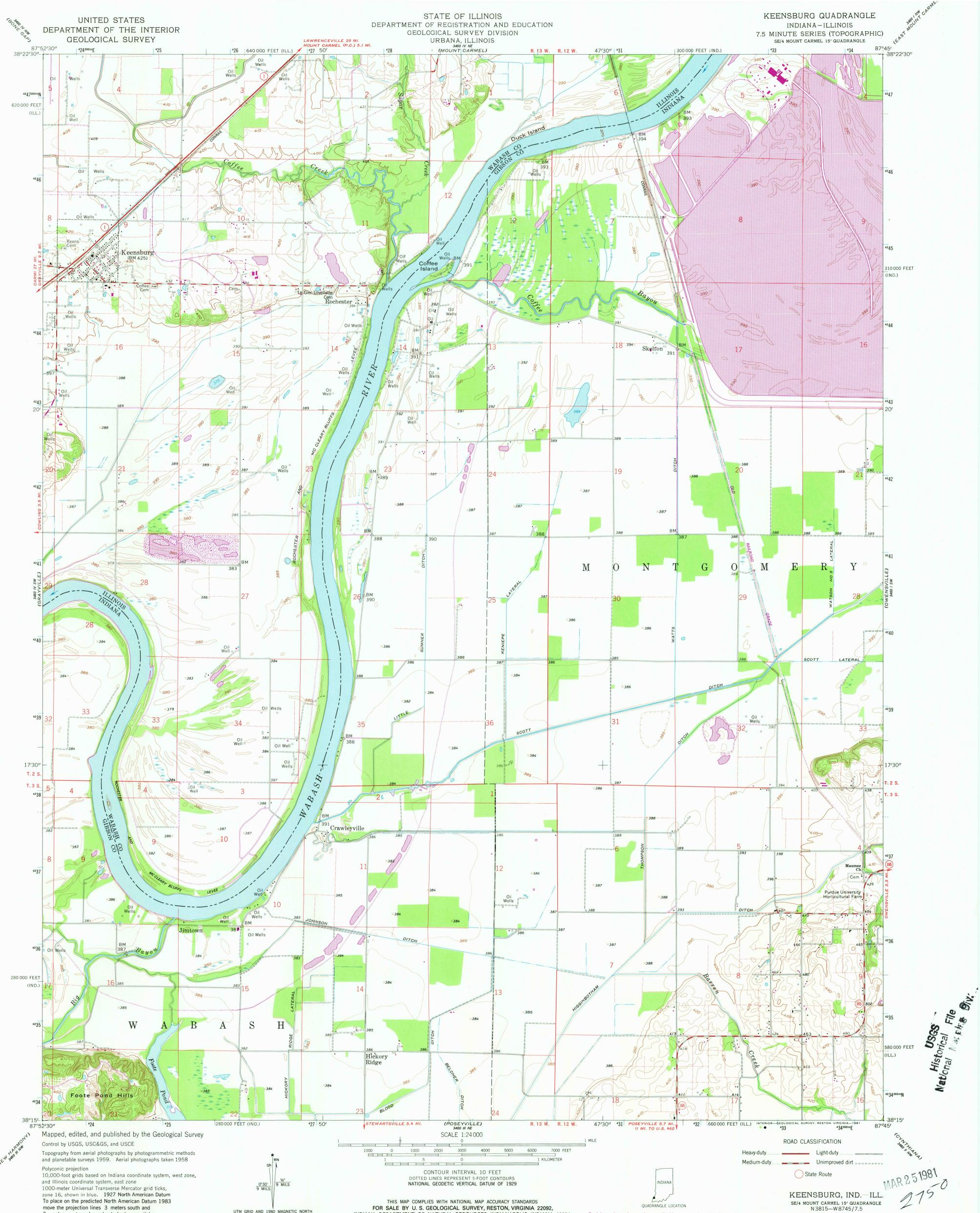
Polyconic projection 10,000-foot grids based on Indiana coordinate system, west zone, and Illinois coordinate system, east zone 1000-meter Universal Transverse Mercator grid ticks, zone 16, shown in blue. 1927 North American Datum To place on the predicted North American Datum 1983 move the projection lines 3 meters south and 3 meters east as shown by dashed corner ticks
