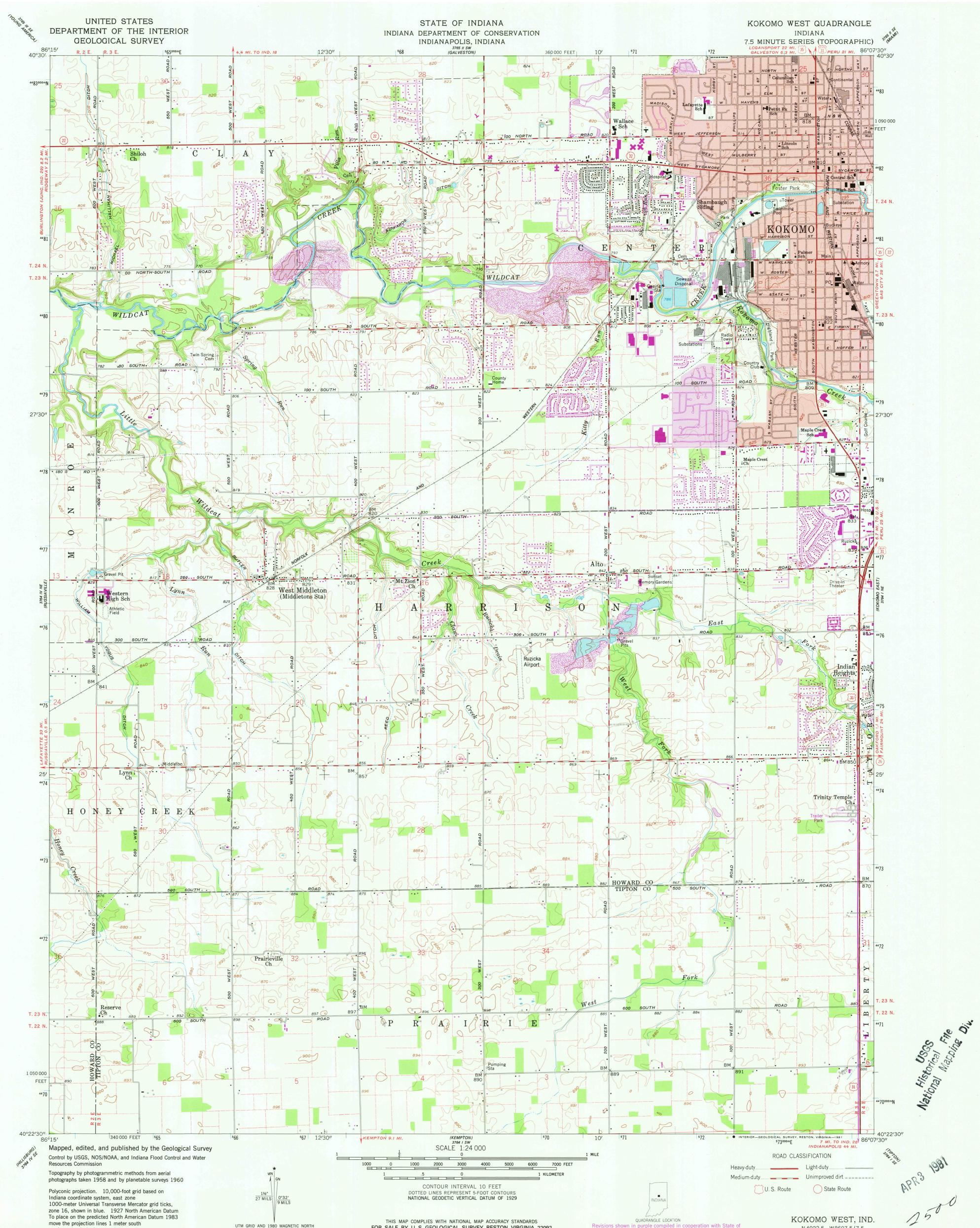
Polyconic projection. 10,000-foot grid based on Indiana coordinate system, east zone 1000-meter Universal Transverse Mercator grid ticks, zone 16, shown in blue. 1927 North American Datum To place on the predicted North American Datum 1983 move the projection lines 1 meter south as shown by dashed corner ticks
