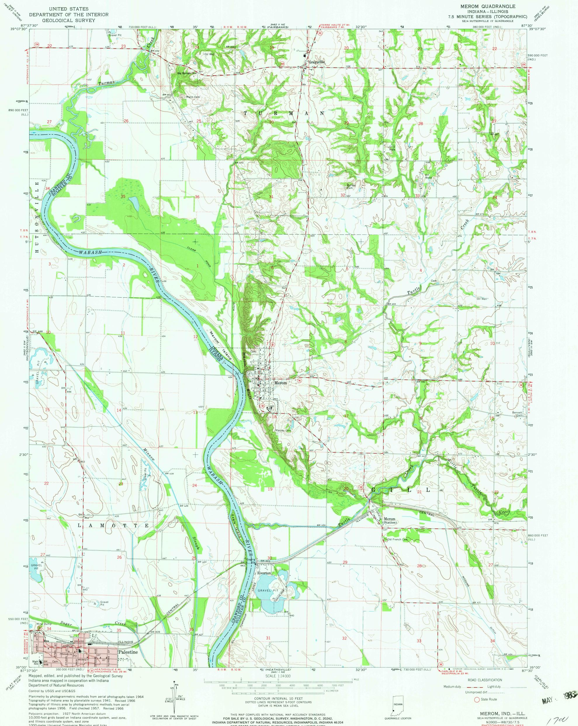
Topography of Indiana area by planetable surveys 1941. Revised 1966 Topography of Illinois area by photogrammetric methods from aerial photographs taken 1956. Field checked 1957. Revised 1966
