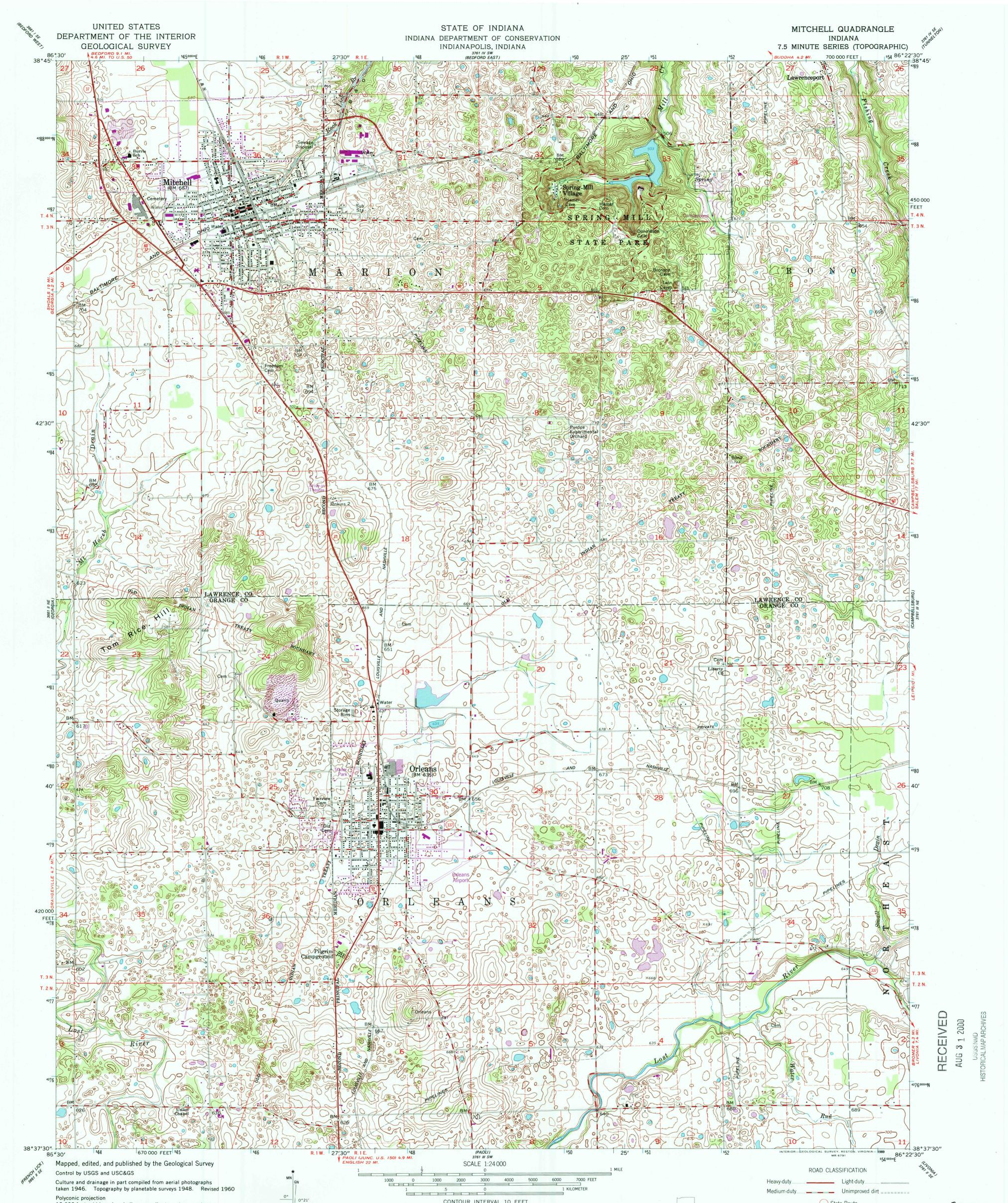
10,000-foot grid based on Indiana coordinate system, west zone 1000-meter Universal Transverse Mercator grid ticks, zone 16, shown in blue. 1927 North American Datum To place on the predicted North American Datum 1983 move the projection lines 3 meters south and 1 meter west as shown by dashed corner ticks
