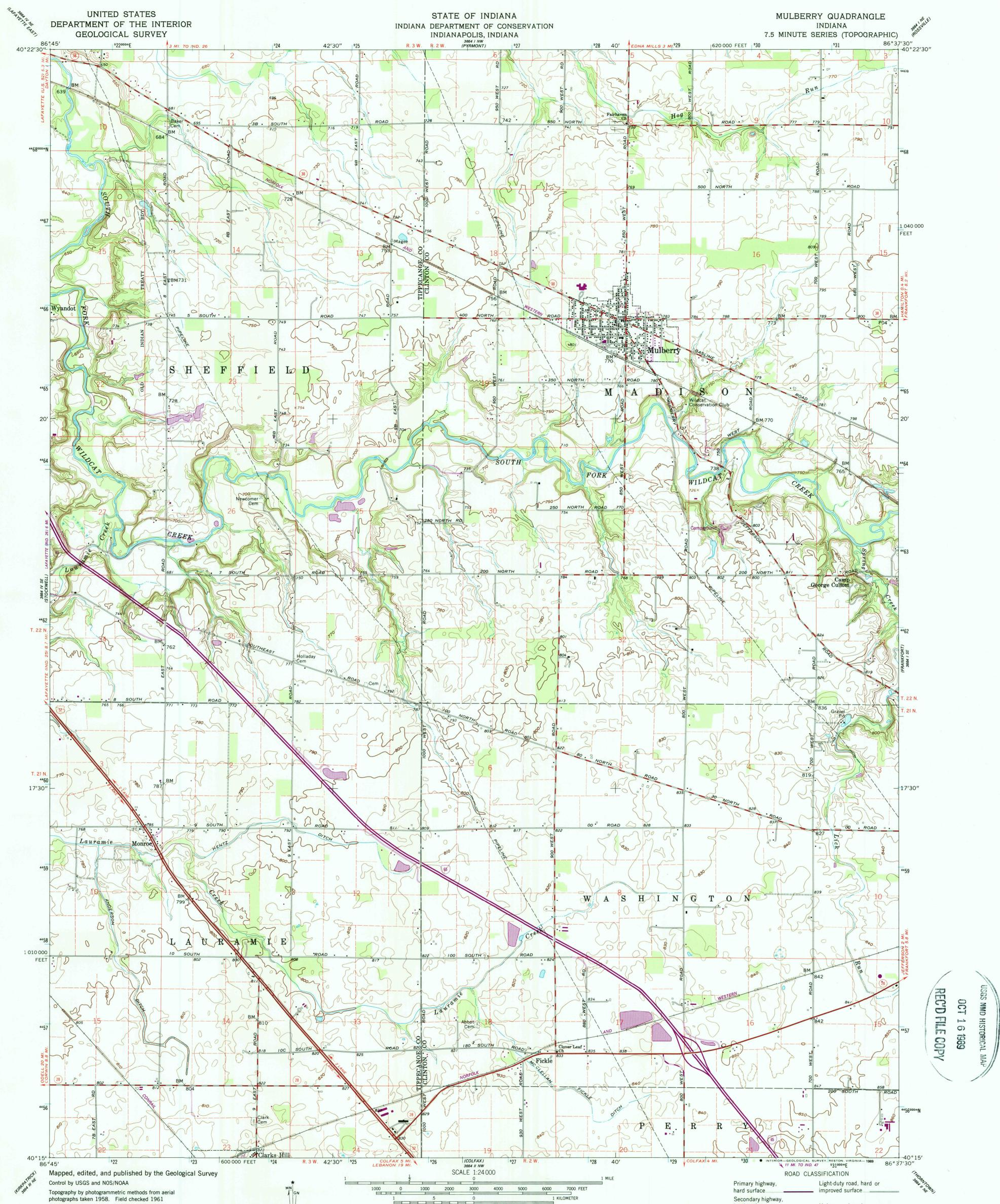
Polyconic projection. 10,000-foot grid based on Indiana coordinate system, west zone 1000-meter Universal Transverse Mercator grid ticks, zone 16, shown in blue. 1927 North American Datum To place on the predicted North American Datum 1983 move the projection lines 1 meter south and 1 meter east as shown by dashed corner ticks 1° 18 MILS 0°12' 4 MILS
