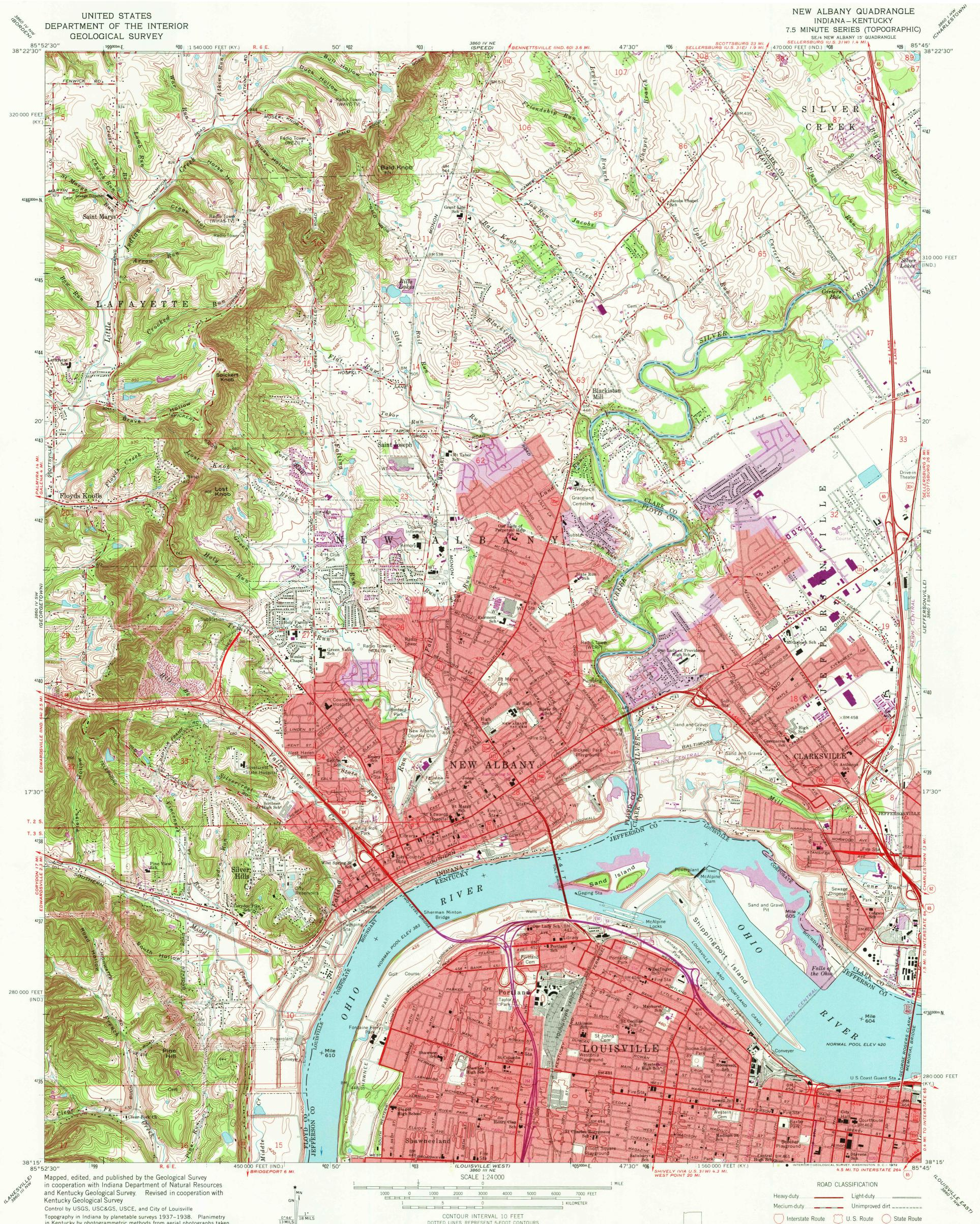
Topography in Indiana by planetable surveys 1937–1938. Planimetry in Kentucky by photogrammetric methods from aerial photographs taken 1949. Topography by planetable surveys 1950. Entire map revised 1965
