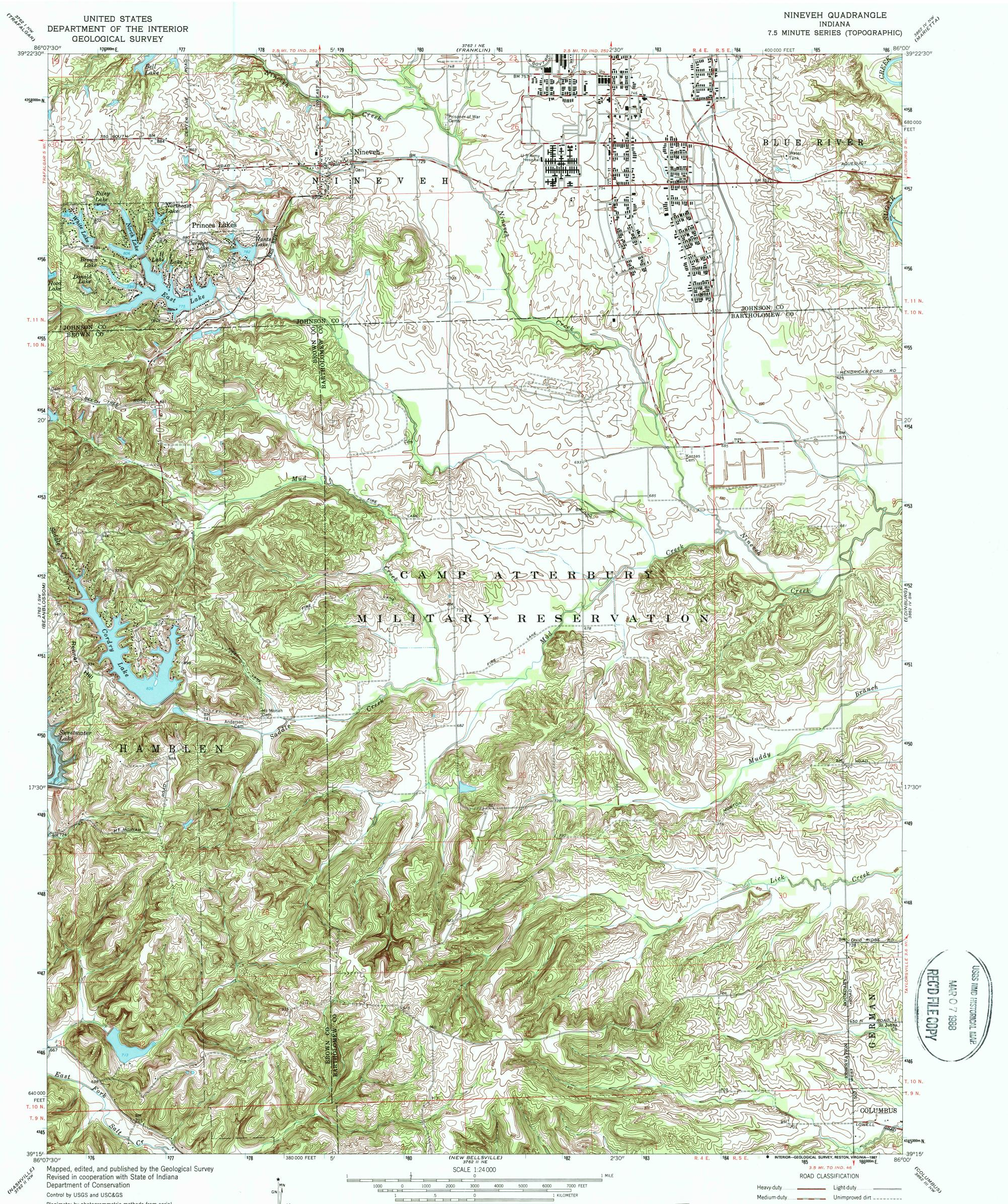
Planimetry by photogrammetric methods from aerial photographs taken 1944. Topography by planetable surveys 1947. Revised 1962
