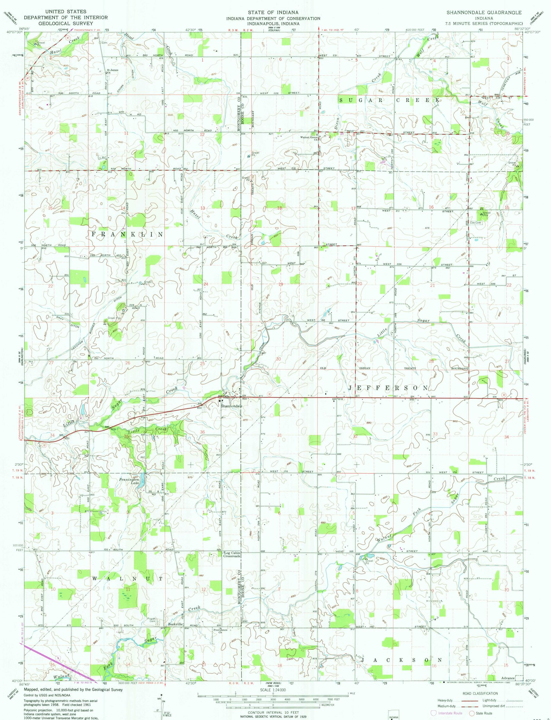
Polyconic projection. 10,000-foot grid based on Indiana coordinate system, west zone 1000-meter Universal Transverse Mercator grid ticks, zone 16, shown in blue. 1927 North American Datum To place on the predicted North American Datum 1983 move the projection lines 1 meter south and 1 meter east as shown by dashed corner ticks
