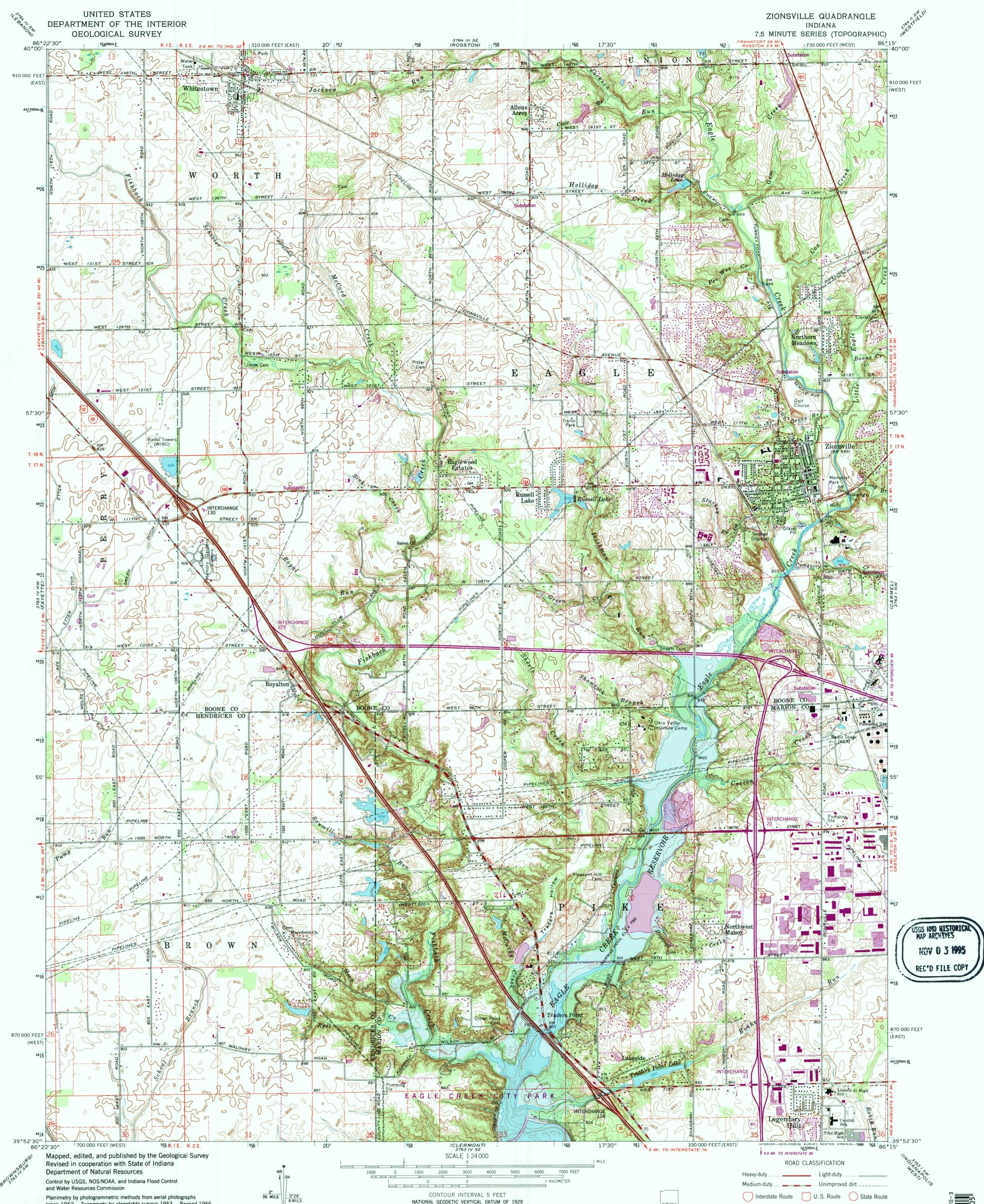
Planimetry by photogrammetric methods from aerial photographs taken 1952. Topography by planetable surveys 1953. Revised 1966 Polyconic projection. 1927 North American Datum 10,000-foot grid ticks based on Indiana coordinate system, west and east zones 1000-meter Universal Transverse Mercator grid ticks, zone 16, shown in blue To place on the predicted North American Datum 1983 to controlled inundation move the projection lines 1 meter south as shown by dashed corner ticks
