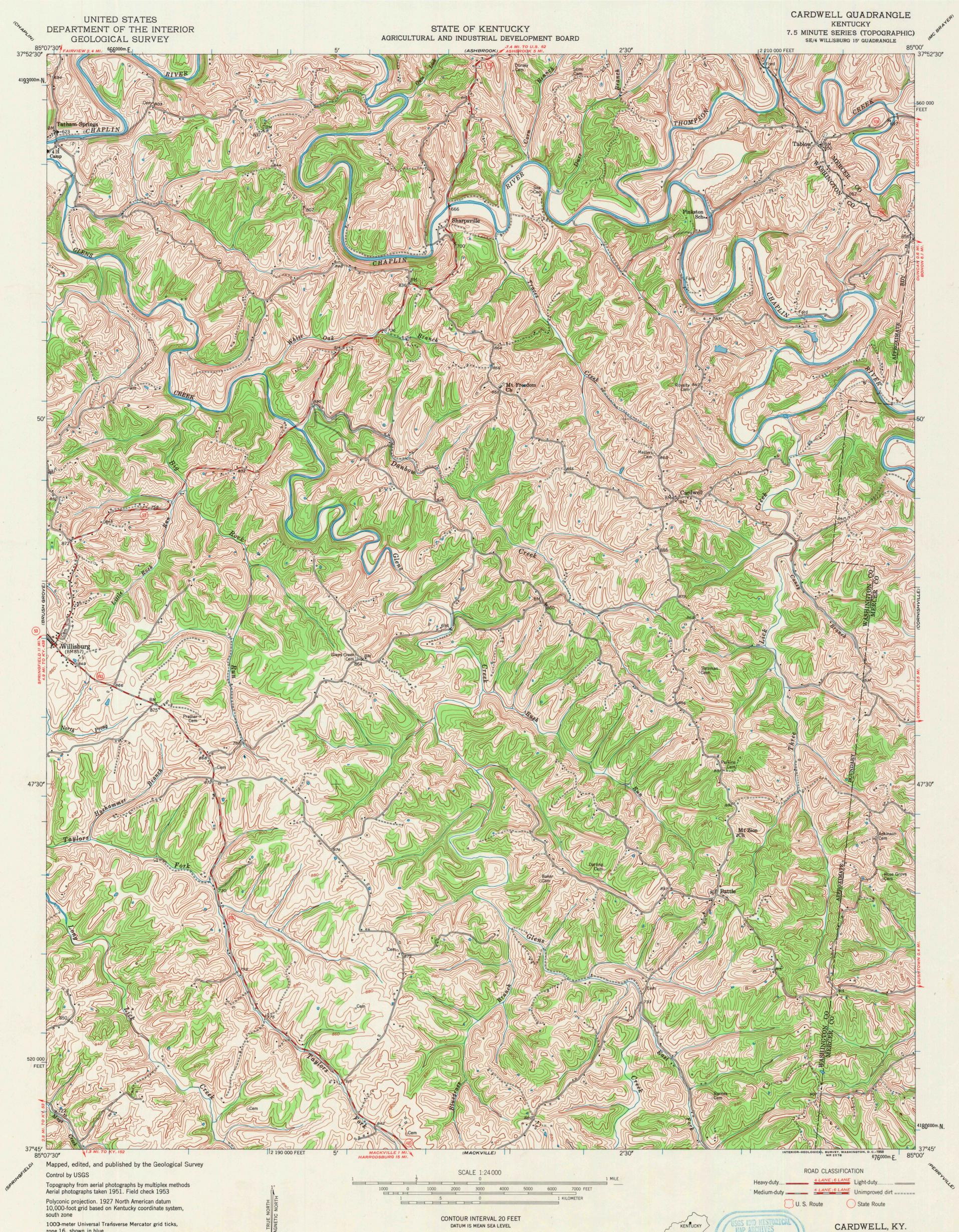
Polyconic projection. 1927 North American datum 10,000-foot grid based on Kentucky coordinate system, south zone
