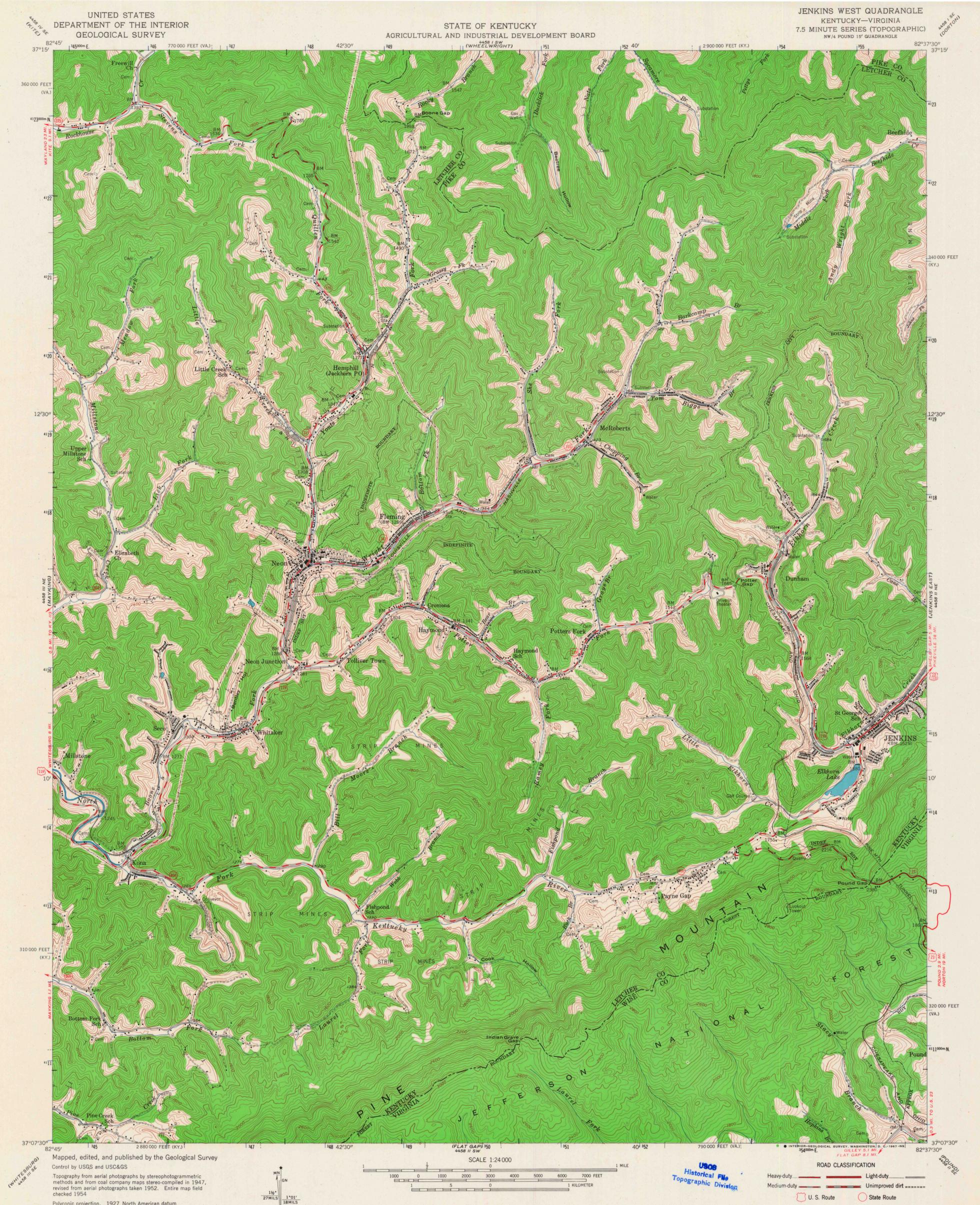
Polyconic projection. 1927 North American datum 10,000-foot grids based on Kentucky coordinate system, south zone and Virginia coordinate system, south zone Contours in strip mine areas from 1952 photography 1000-meter Universal Transverse Mercator grid ticks, zone 17, shown in blue
