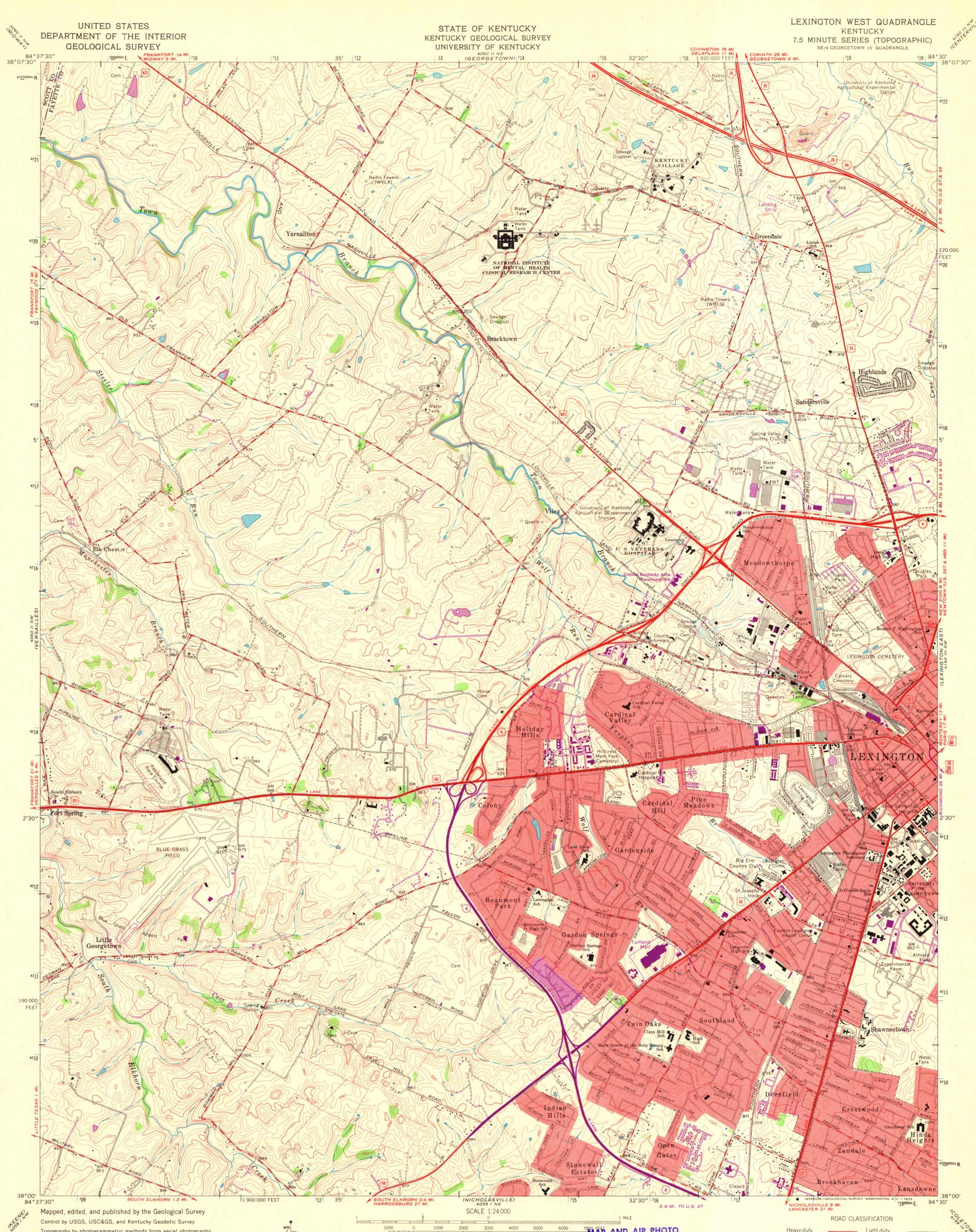
Topography by photogrammetric methods from aerial photographs taken 1949. Field checked 1950. Revised 1965
