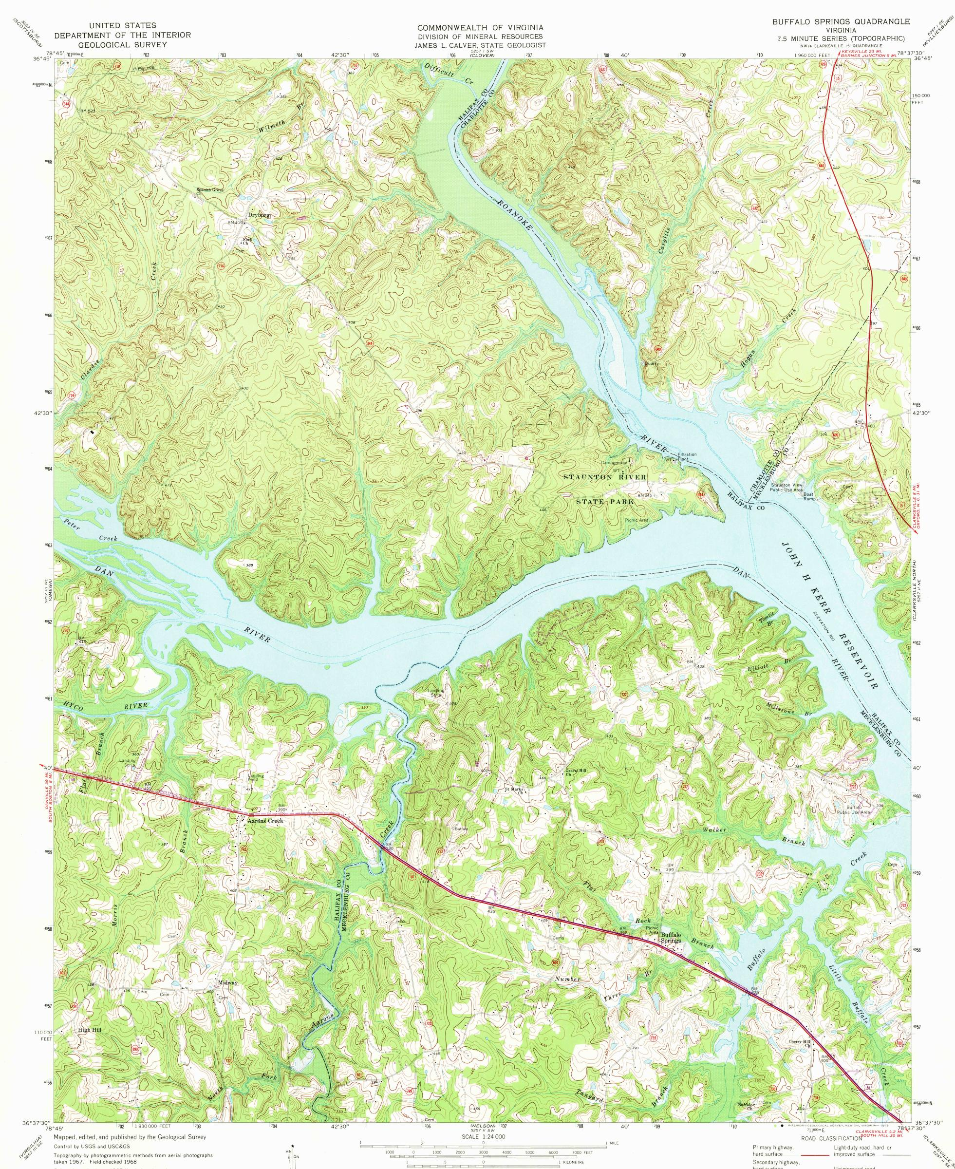
Polyconic projection. 1927 North American datum 10,000-foot grid based on Virginia coordinate system, south zone 1000-metre Universal Transverse Mercator grid ticks, zone 17, shown in blue
