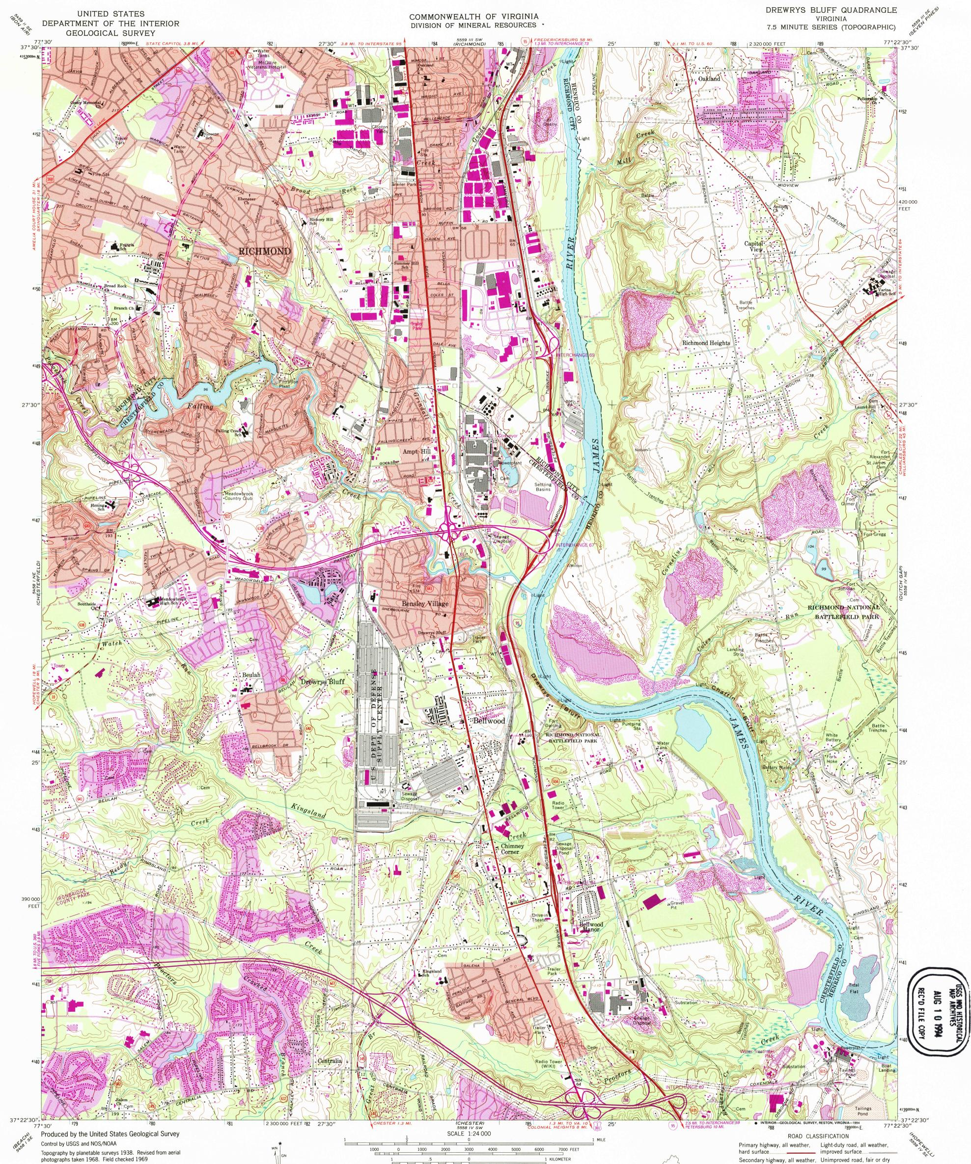
Projection and 10,000-foot grid ticks: Virginia coordinate system, south zone (Lambert conformal conic) 1000-meter Universal Transverse Mercator grid ticks, zone 18, shown in blue 1927 North American Datum (NAD 27)
