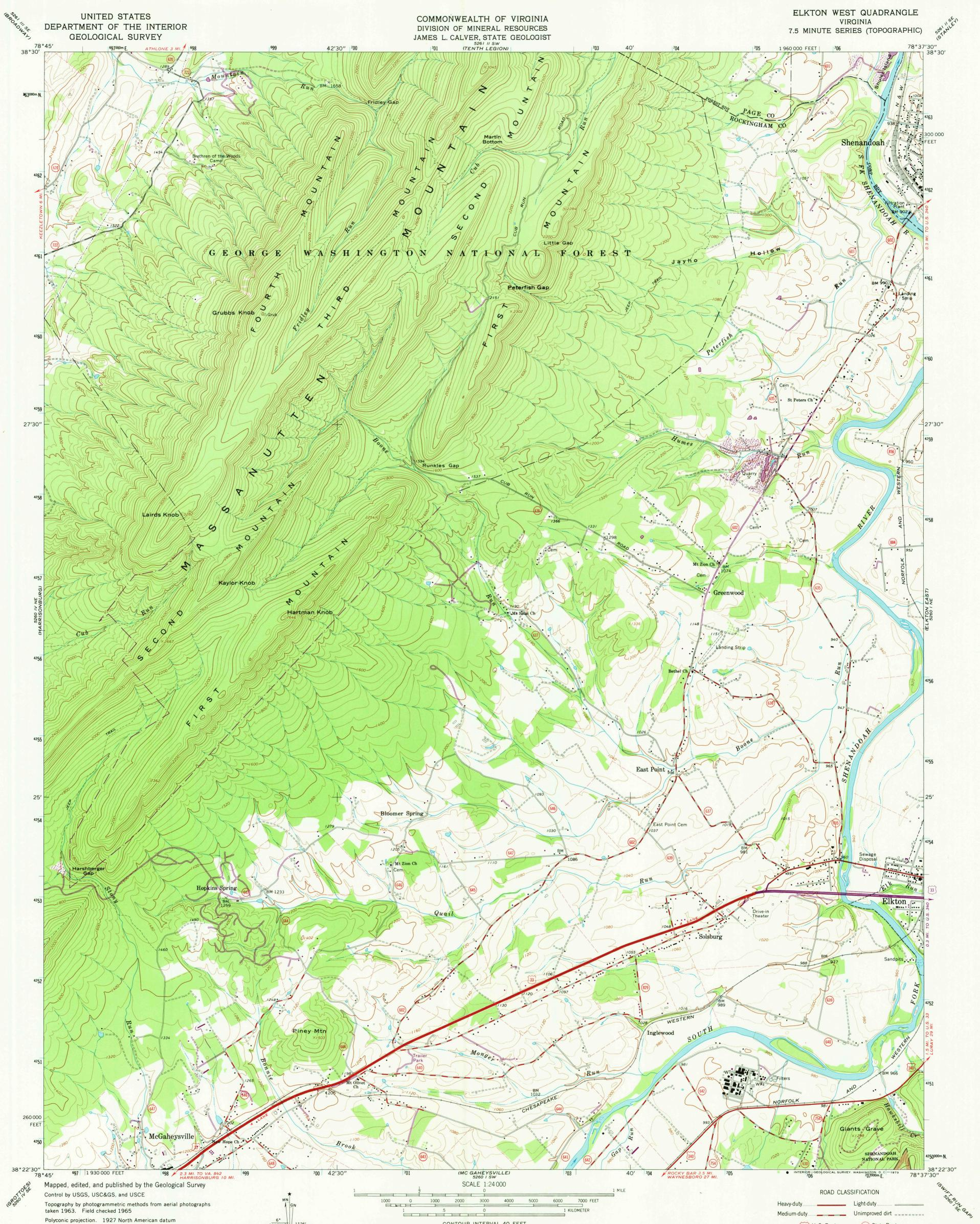
10,000-foot grid based on Virginia coordinate system, north zone 1000-meter Universal Transverse Mercator grid ticks, zone 17, shown in blue
