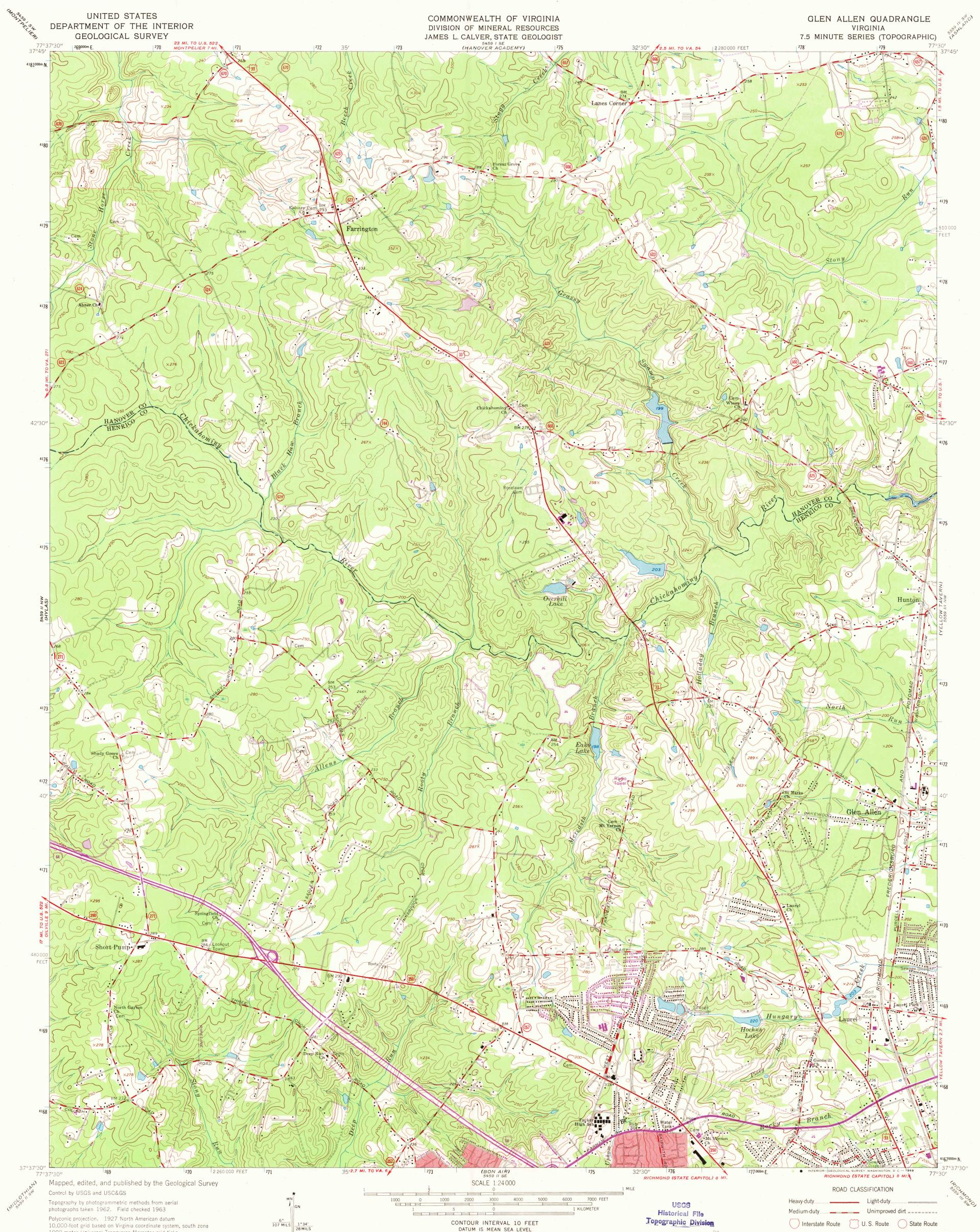
10,000-foot grid based on Virginia coordinate system, south zone 1000-meter Universal Transverse Mercator grid ticks, zone 18, shown in blue
