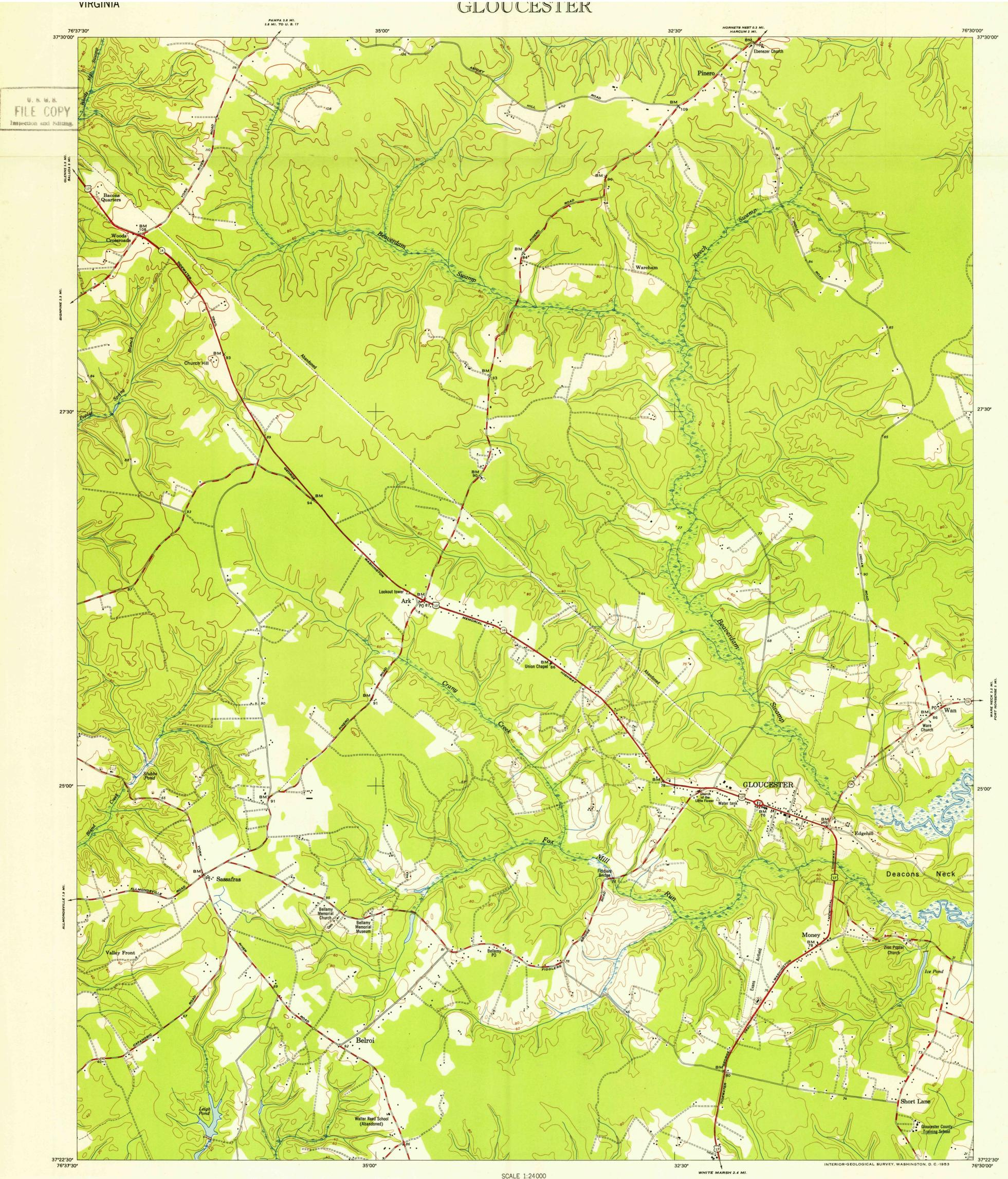
Published by the Army Map Service, Corps of Engineers, U. S. Army, Washington, D. C. Compiled in 1951 by the Coast and Geodetic Survey, U. S. Department of Commerce, by photogrammetric (Reading Plotter) methods from aerial photography dated March 1948 and field surveys of June, 1944. Horizontal and vertical control by USC&GS. Map not field checked.
