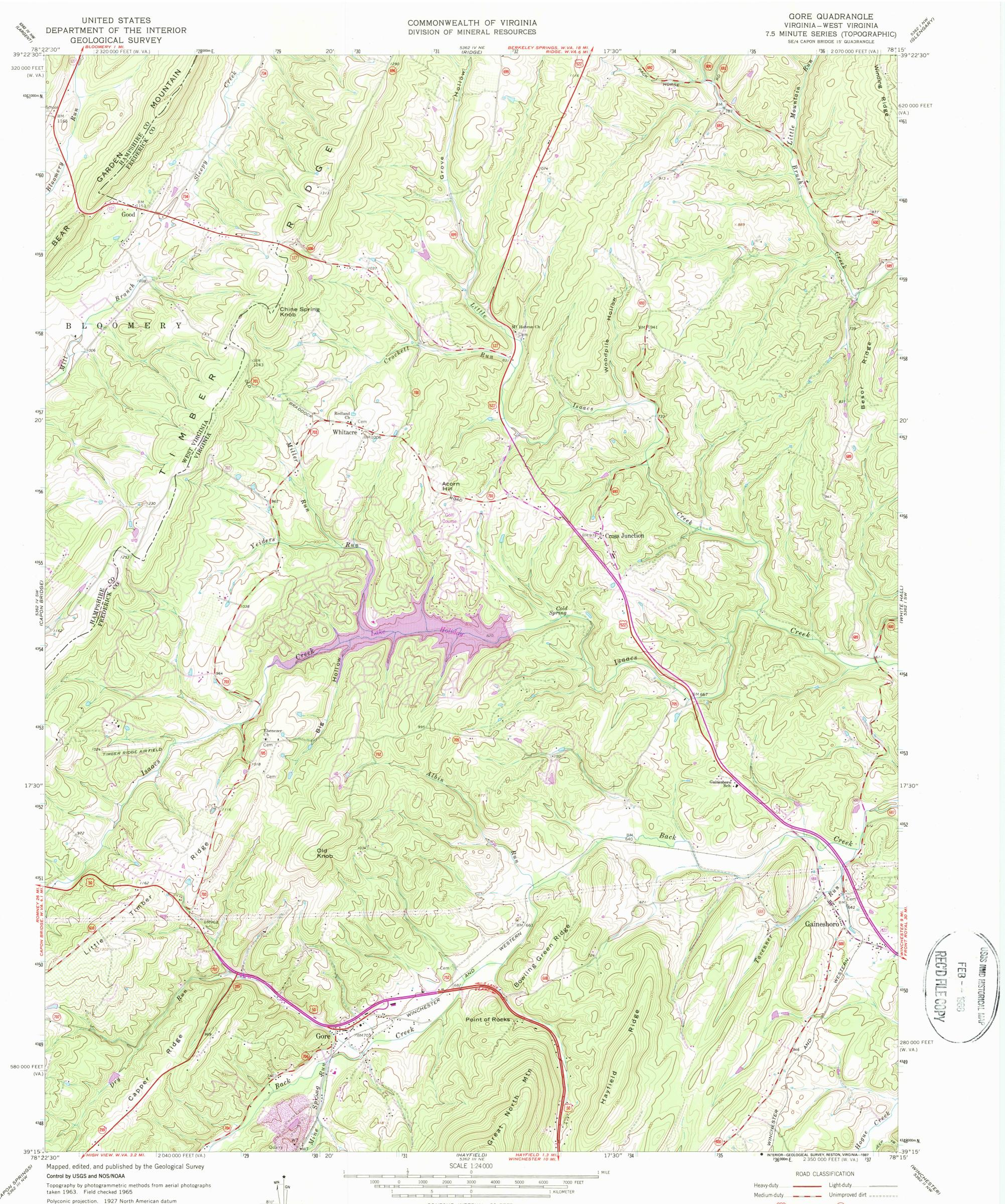
10,000-foot grids based on Virginia coordinate system, north zone, and West Virginia coordinate system, north zone 1000-meter Universal Transverse Mercator grid ticks, zone 17, shown in blue To place on the predicted North American Datum 1983 move the projection lines 7 meters south and 23 meters west as shown by dashed corner ticks Fine red dashed lines indicate selected fence and field lines where generally visible on aerial photographs. This information is unchecked
