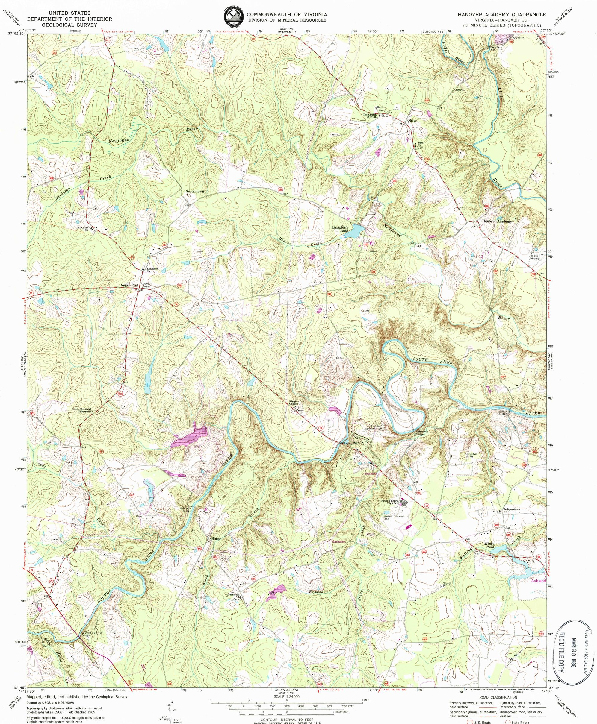
Polyconic projection. 10,000-foot grid ticks based on Virginia coordinate system, south zone 1000-meter Universal Transverse Mercator grid ticks, zone 18, shown in blue 1927 North American Datum To place on the predicted North American Datum 1983 move the projection lines 10 meters south and 26 meters west as shown by dashed corner ticks
