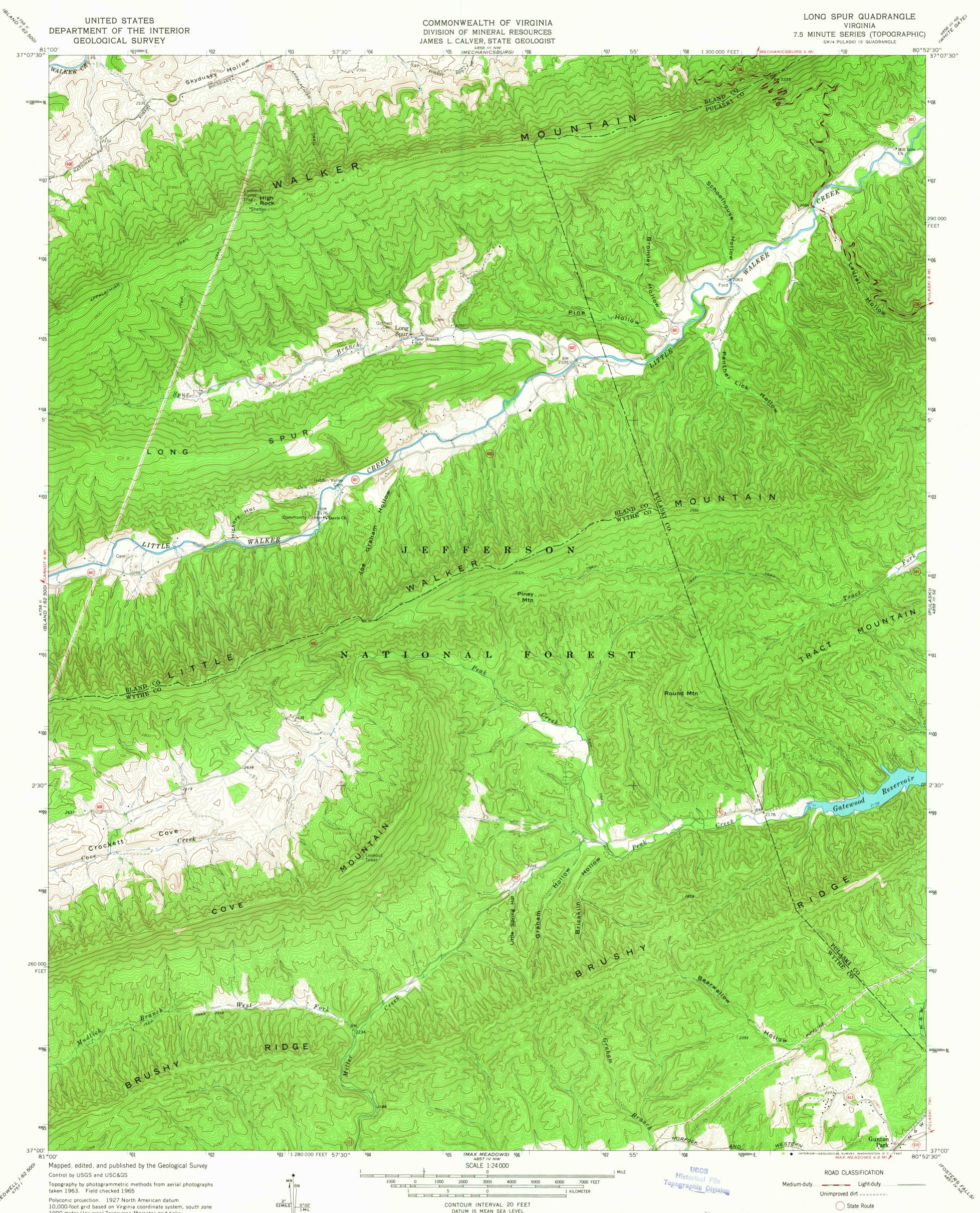
10,000-foot grid based on Virginia coordinate system, south zone 1000-meter Universal Transverse Mercator grid ticks, zone 17, shown in blue
