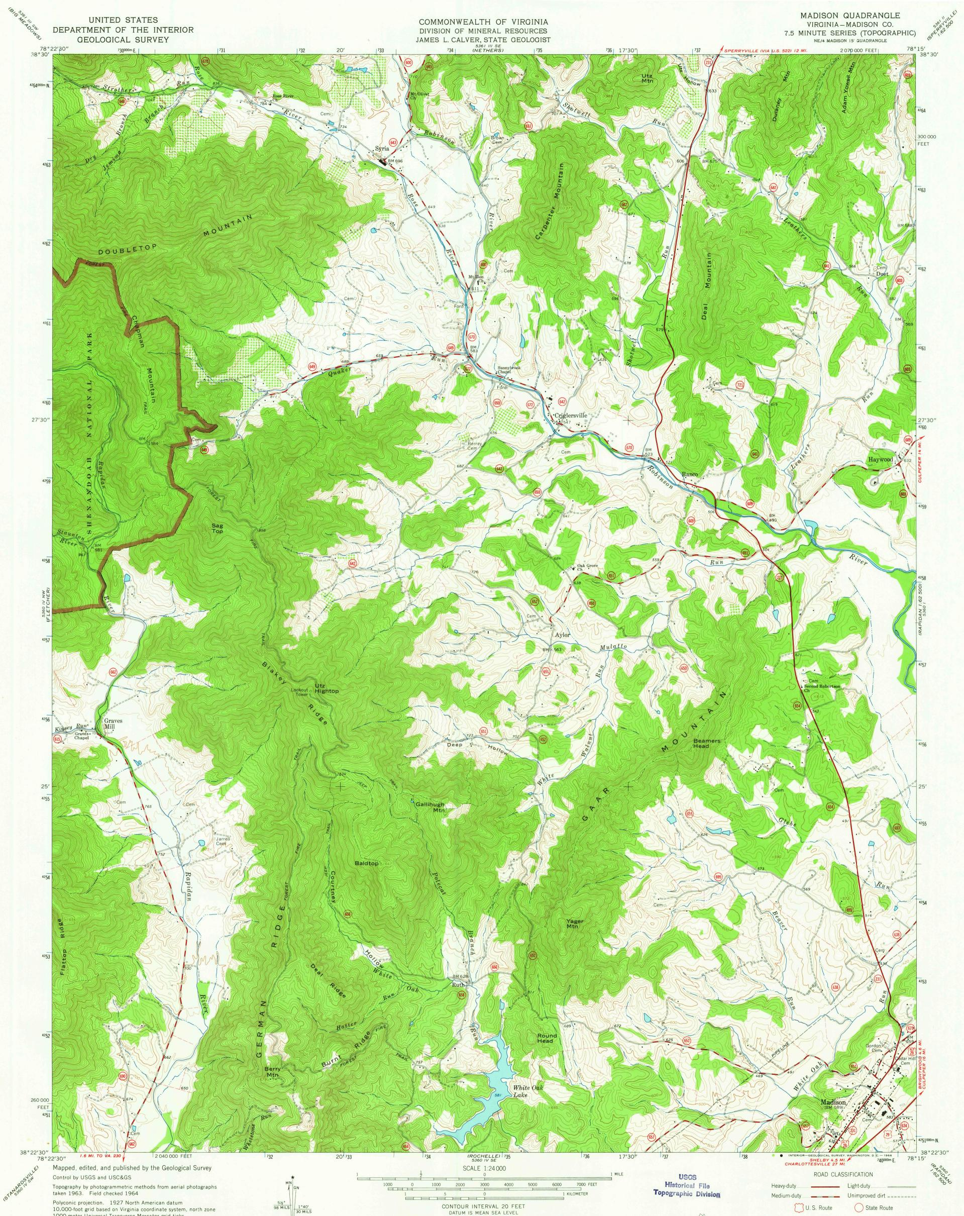
Polyconic projection. 1927 North American datum 10,000-foot grid based on Virginia coordinate system, north zone 1000-meter Universal Transverse Mercator grid ticks, zone 17, shown in blue
