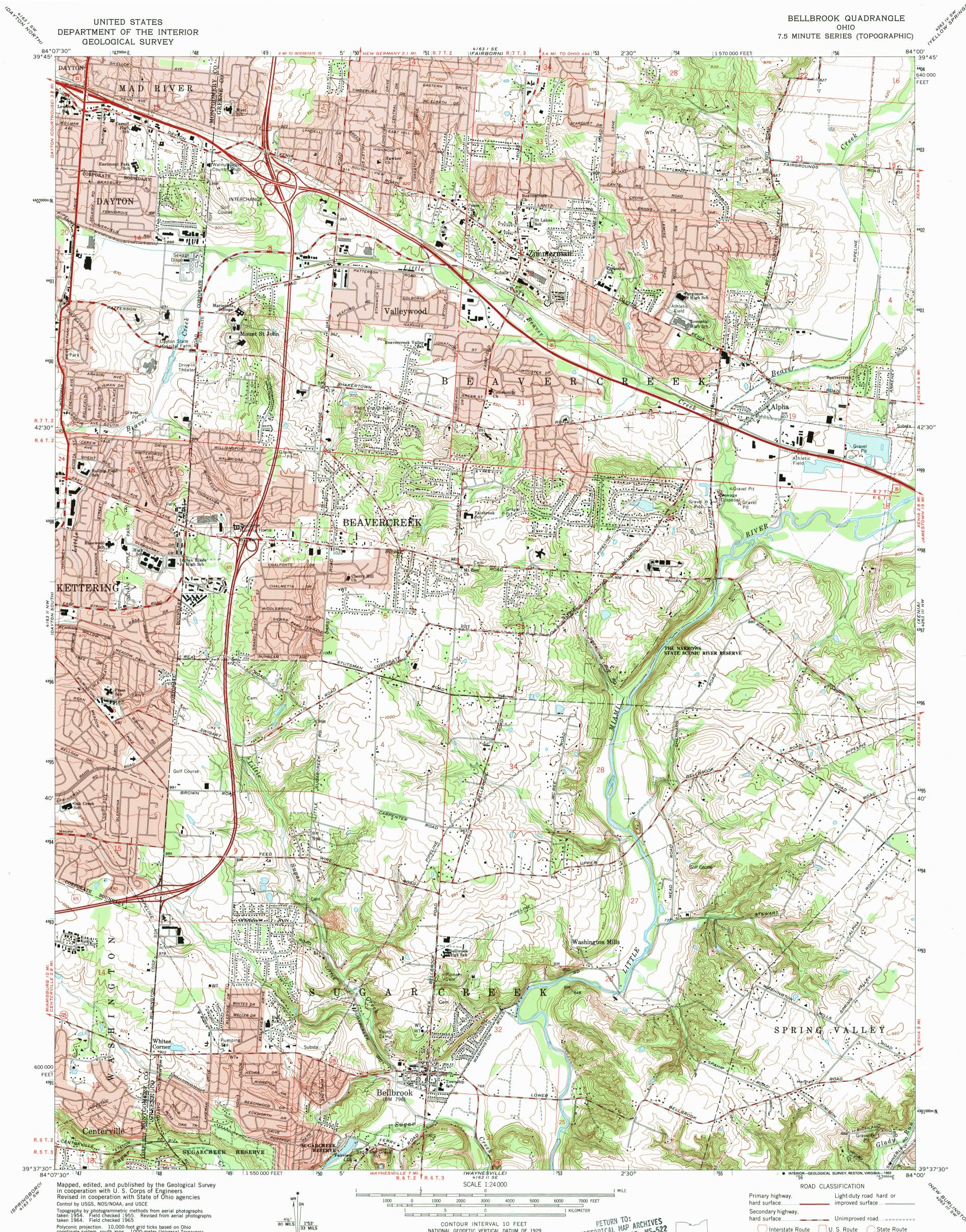
Polyconic projection. 10,000-foot grid ticks based on Ohio coordinate system, south zone. 1000-meter Universal Transverse Mercator grid ticks, zone 16, shown in blue. 1927 North American Datum. The difference between 1927 North American Datum and North American Datum of 1983 (NAD 83) for 7.5-minute intersections is given in USGS Bulletin 1875. The NAD 83 is shown by dashed corner ticks
