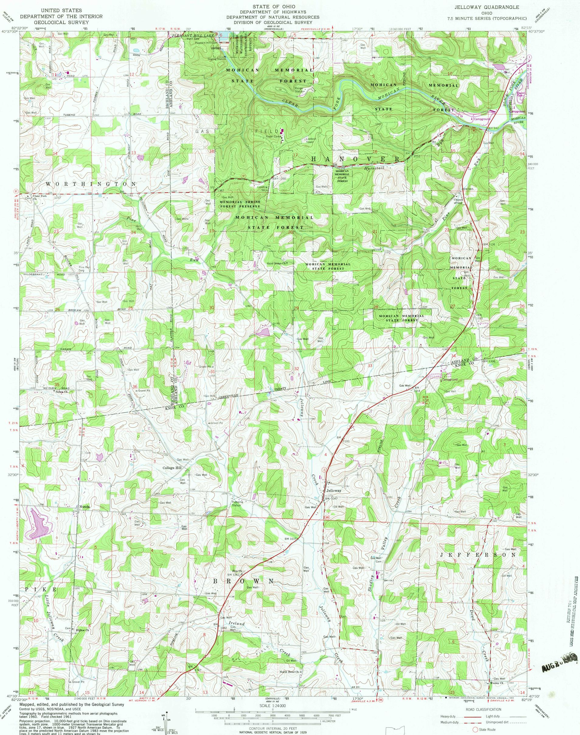
Polyconic projection. 10,000-foot grid ticks based on Ohio coordinate system, north zone. 1000-meter Universal Transverse Mercator grid ticks, zone 17, shown in blue. 1927 North American Datum. To place on the predicted North American Datum 1983 move the projection lines 3 meters south and 11 meters west as shown by dashed corpor ticks dashed corner ticks
