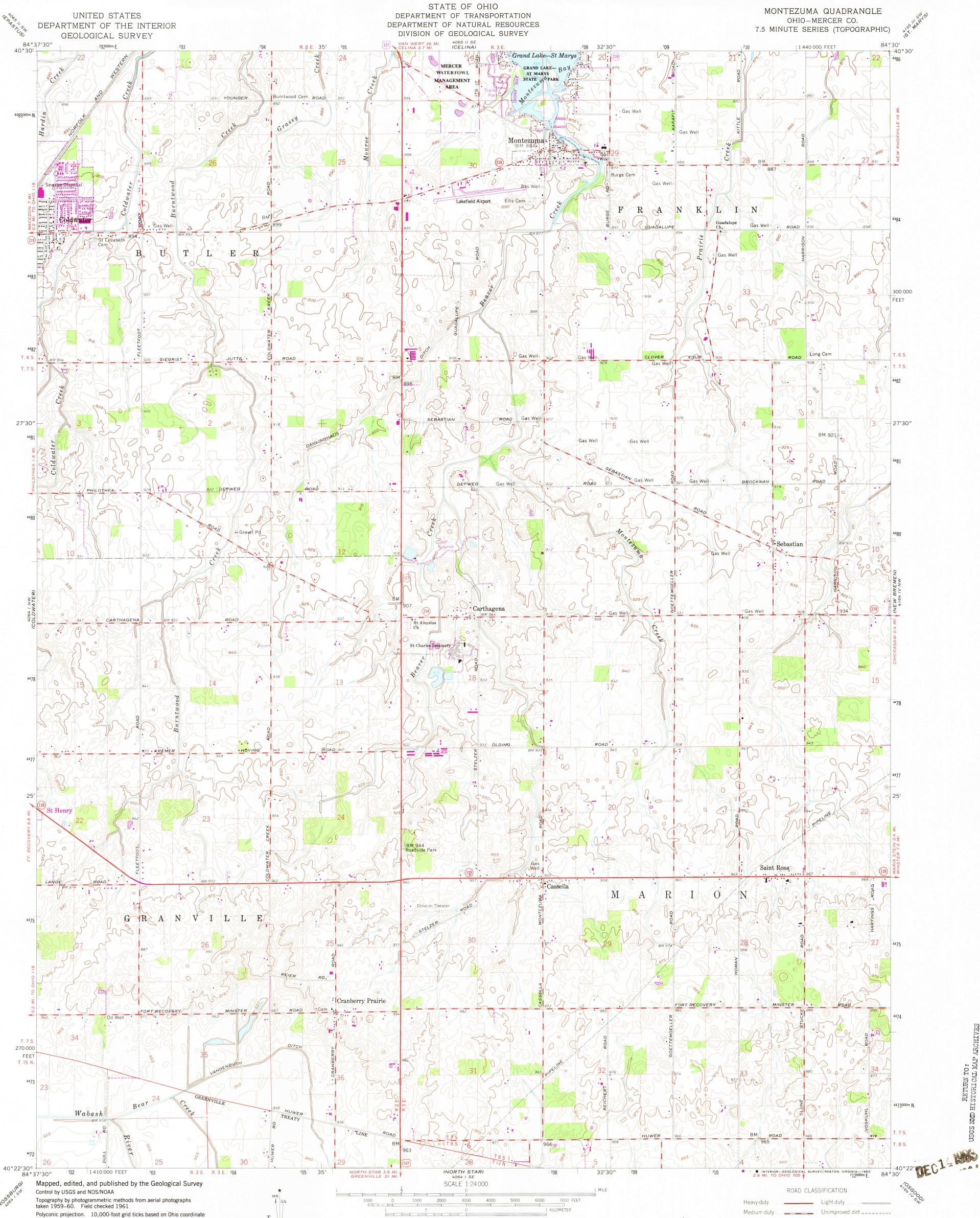
system, north zone. 1000-meter Universal Transverse Mercator grid ticks, zone 16, shown in blue. 1927 North American Datum To place on the predicted North American Catum 1983 move the projection lines 1 meter south and 5 meters west as shown by dashed corner ticks
