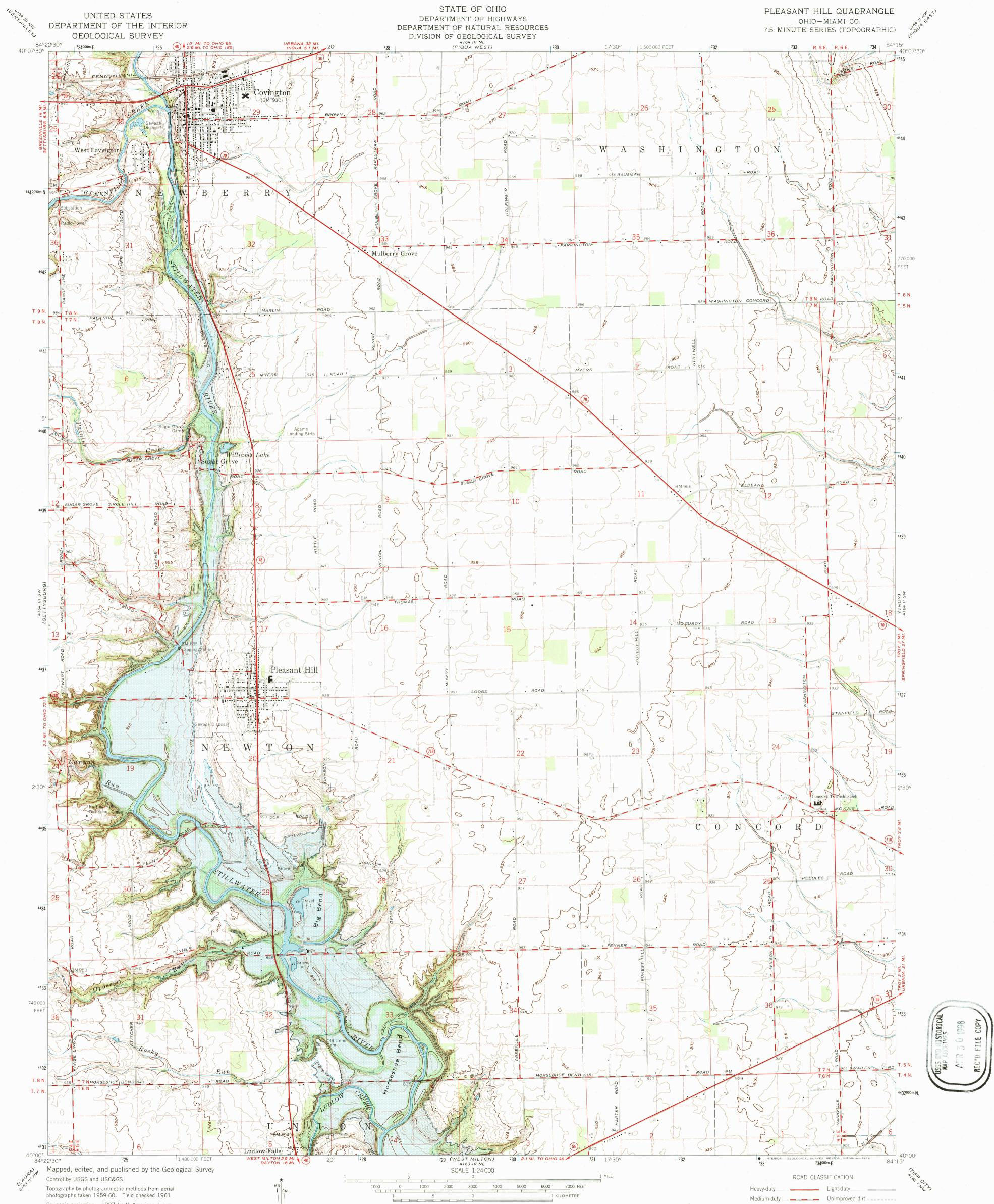
Polyconic projection. 1927 North American datum 10,000-foot grid based on Ohio coordinate system, south zone 1000-metre Universal Transverse Mercator grid ticks, zone 16, shown in blue
