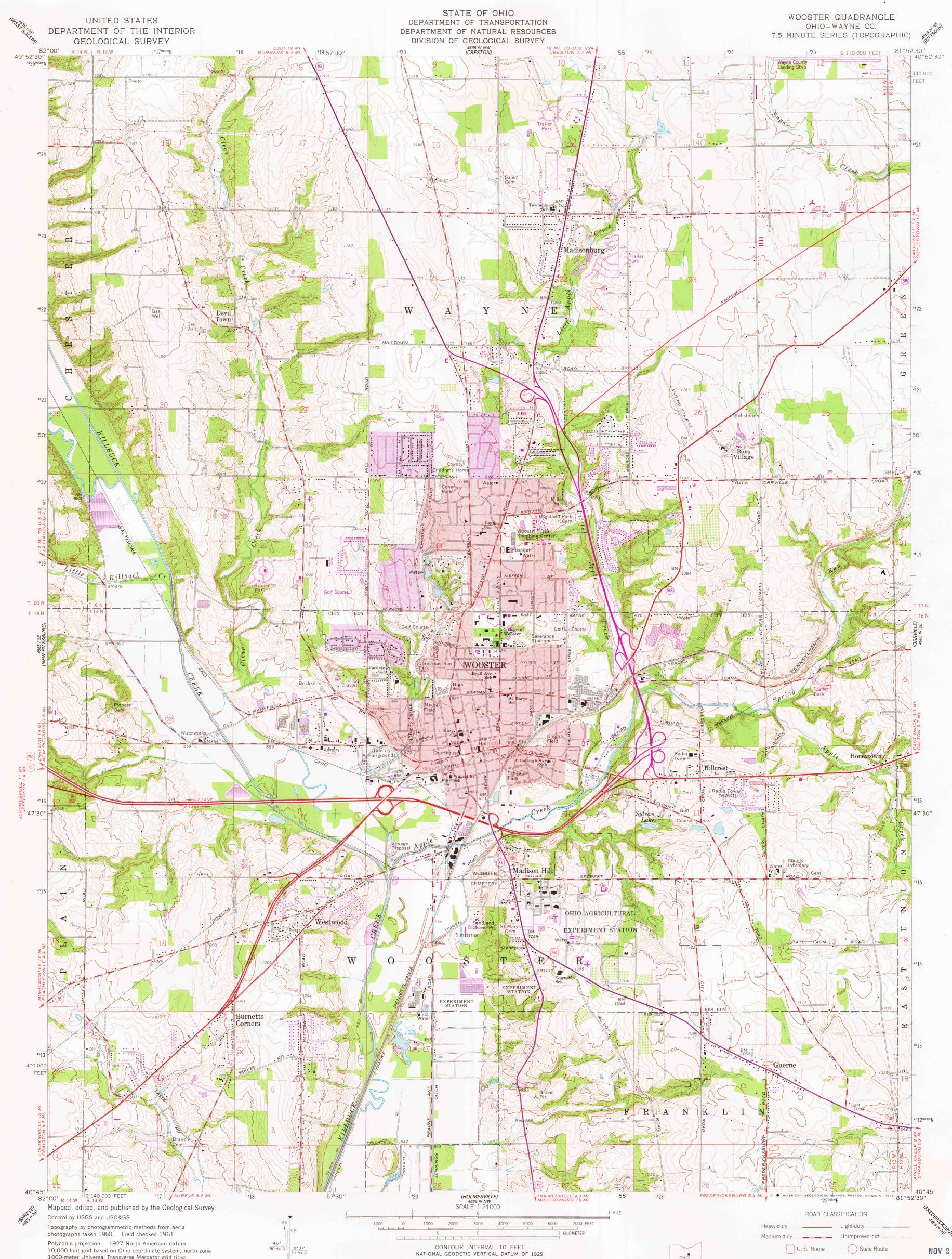
Polyconic projection. 1927 North American datum 10,000-foot grid based on Ohio coordinate system, north zone 1000-meter Universal Transverse Mercator grid ticks, zone 17, shown in blue
