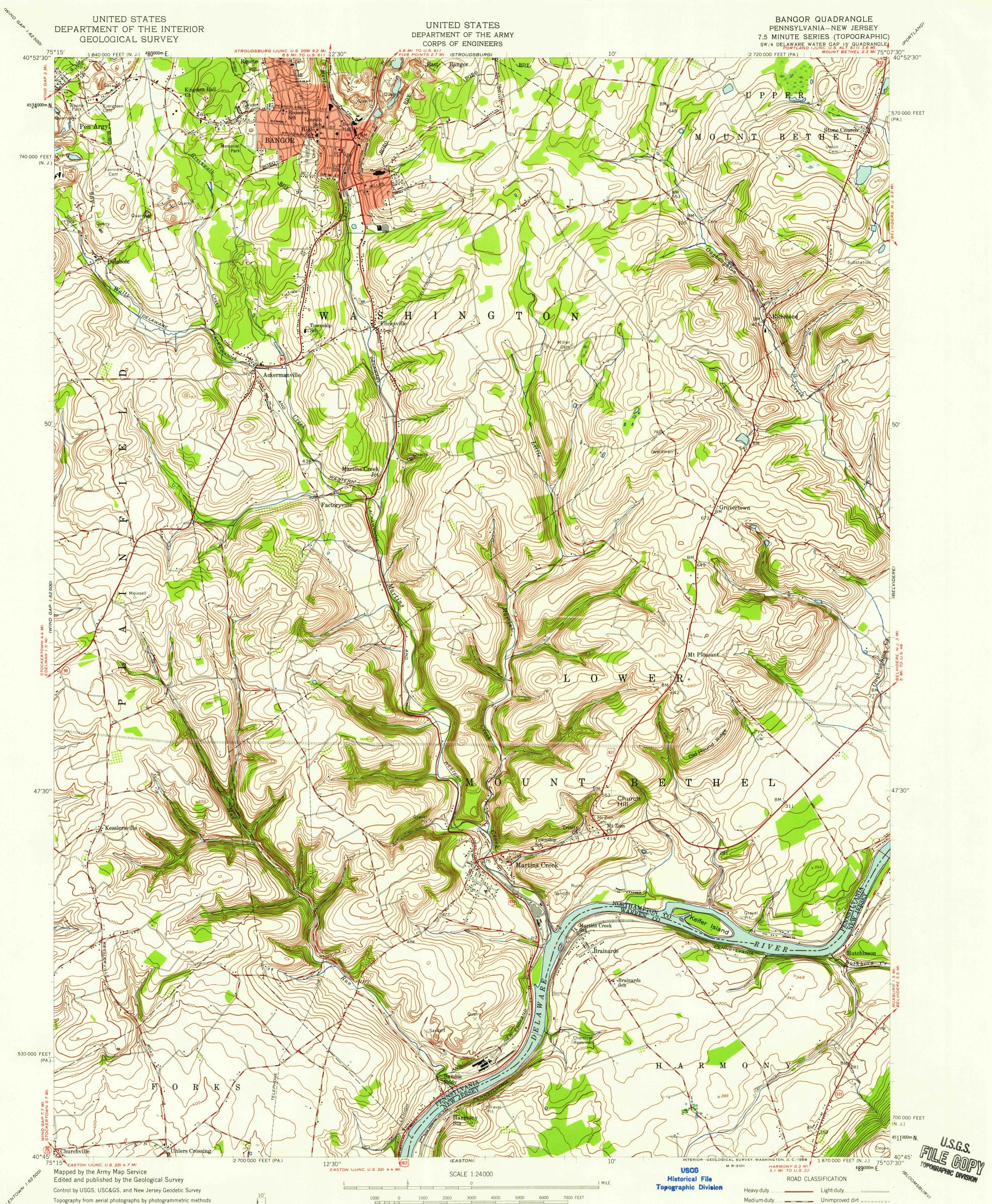
Aerial photographs taken 1942. Field check 1943 Culture revised by the Geological Survey 1956 Polyconic projection. 1927 North American datum 10,000-foot grids based on Pennsylvania coordinate system, south zone, and on New Jersey coordinate system 1000-meter Universal Transverse Mercator grid ticks, zone 18, shown in blue
