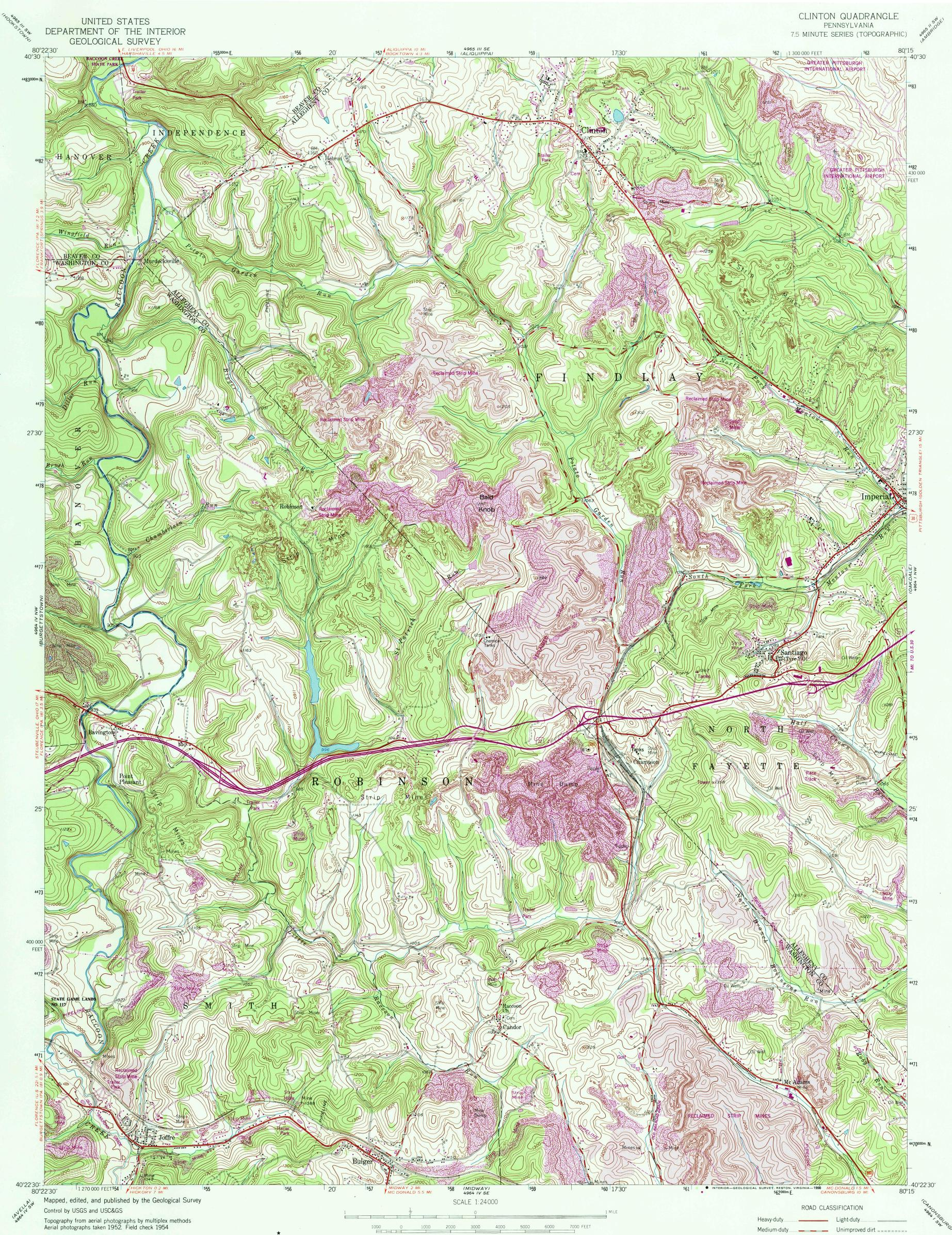
Polyconic projection. 1927 North American datum 10,000-foot grid based on Pennsylvania coordinate system, south zone 1000-meter Universal Transverse Mercator grid ticks, zone 17, shown in blue To place on the predicted North American Datum 1983 move the projection lines 4 meters south and 17 meters west as shown by dashed corner ticks There may be private inholdings within the boundaries of the National or State reservations shown on this map
