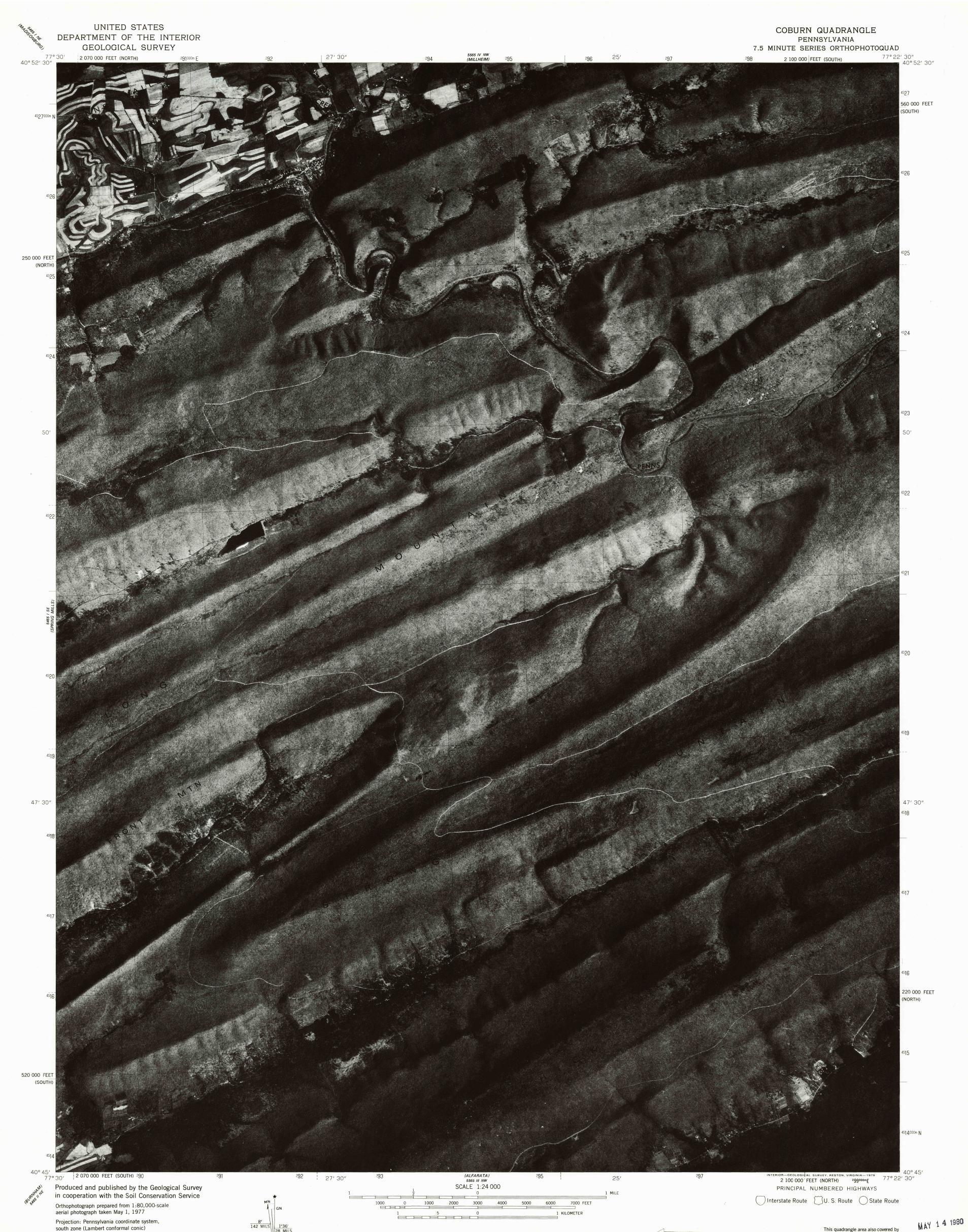
Projection: Pennsylvania coordinate system, south zone (Lambert conformal conic) 10,000-foot grid ticks based on Pennsylvania coordinate system, south and north zones 1000-meter Universal Transverse Mercator grid, zone 18. 1927 North American datum Photoimagery rectified by automatic correlation
