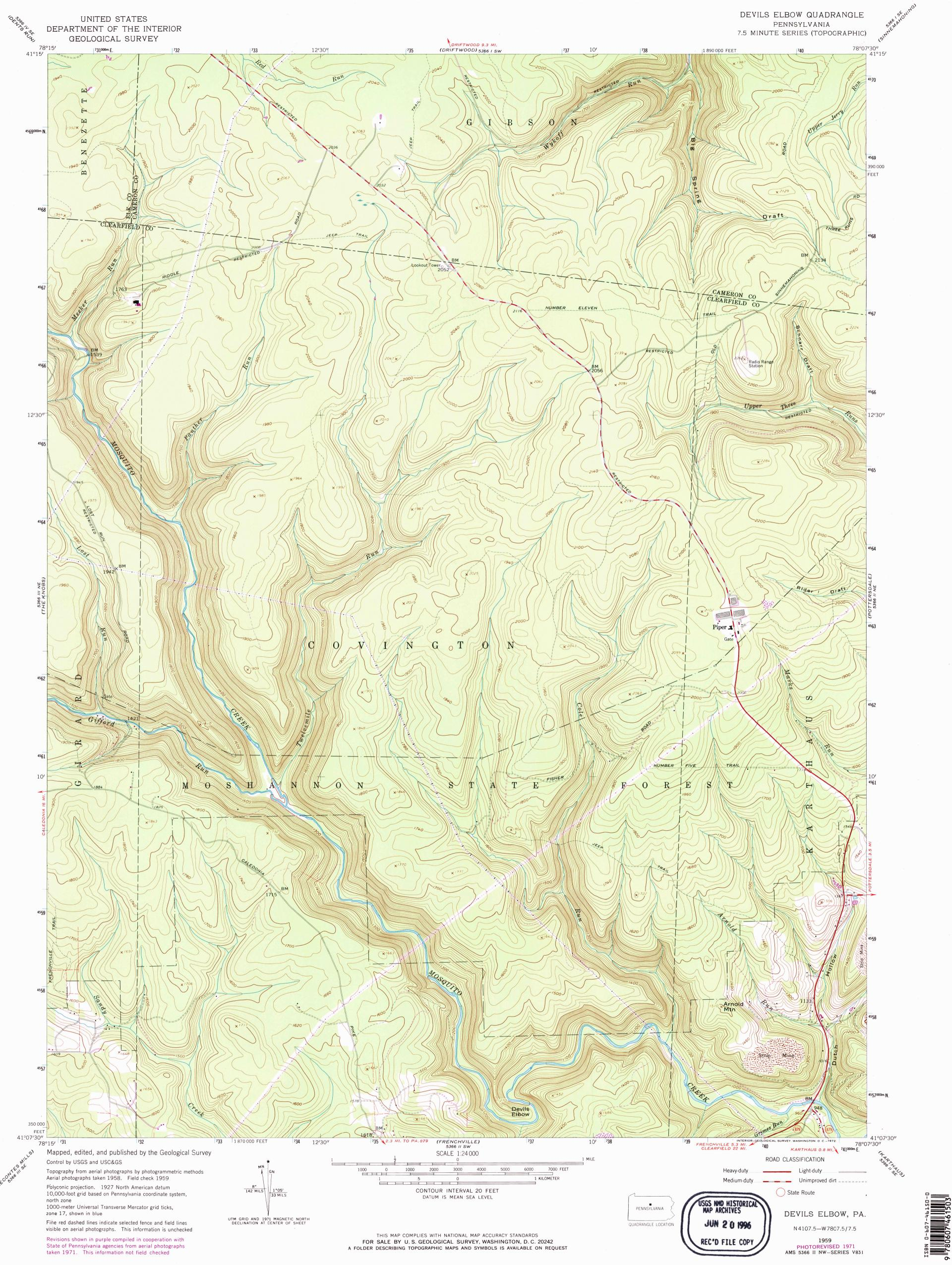
Polyconic projection. 1927 North American datum 10,000-foot grid based on Pennsylvania coordinate system, north zone 1000-meter Universal Transverse Mercator grid ticks, zone 17, shown in blue
