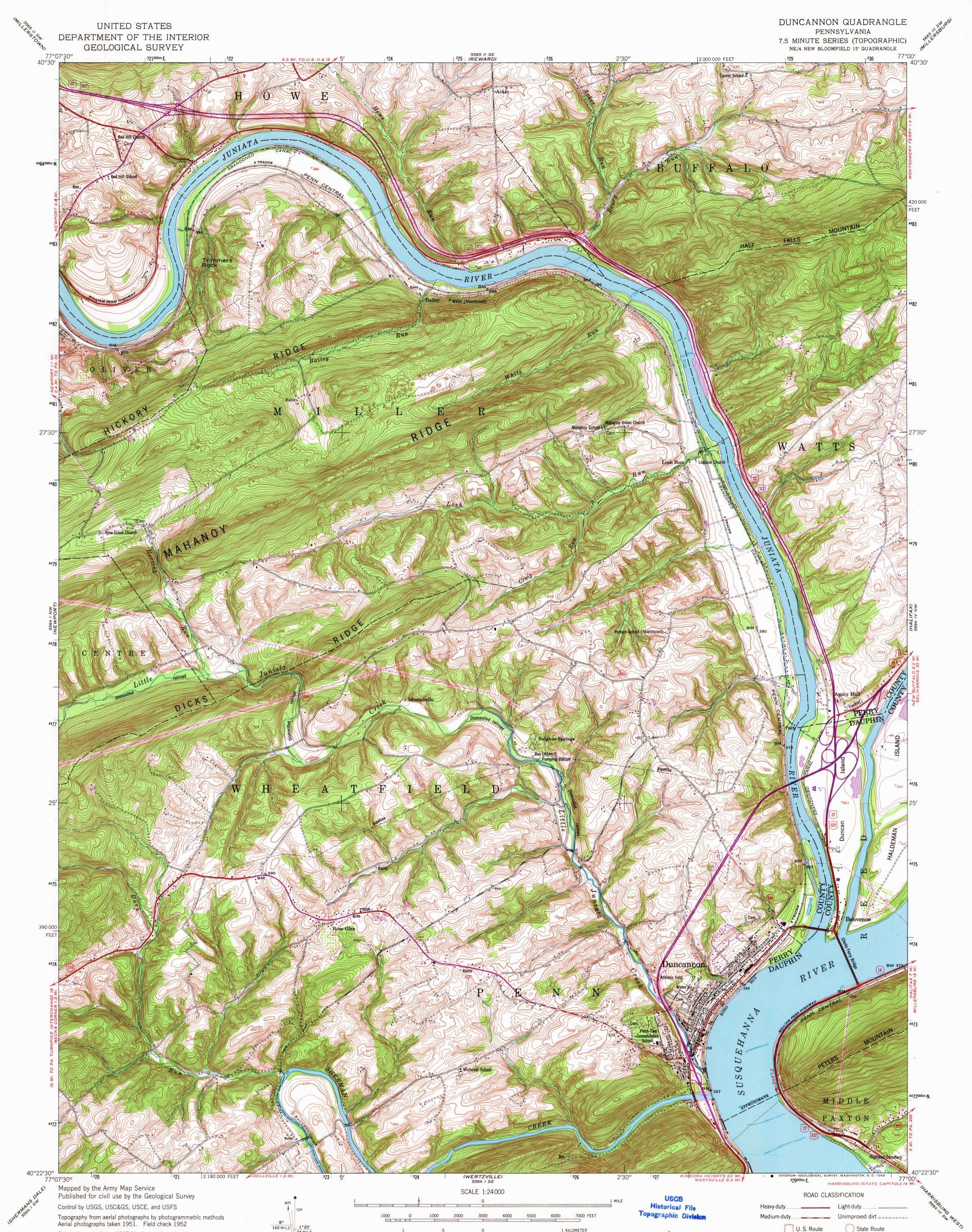
Aerial photographs taken 1951. Field check 1952 Polyconic projection. 1927 North American datum 10,000-foot grid based on Pennsylvania coordinate system, south zone 1000-meter Universal Transverse Mercator grid ticks, zone 18, shown in blue Revisions shown in purple compiled by Geological Survey in cooperation with State of Pennsylvania agencies, from aerial
