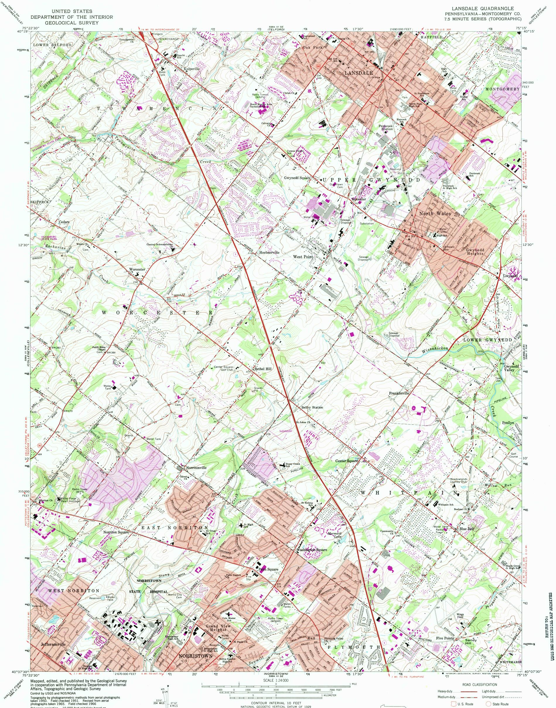
photographs taken 1965. Field checked 1966 Polyconic projection. 10,000-foot grid ticks based on Pennsylvania coordinate system, south zone 1000-meter Universal Transverse Mercator grid ticks, zone 18, shown in blue. 1927 North American Datum To place on the predicted North American Datum 1983 move the projection lines 6 meters south and 21 meters used a shown by deshed access ticks 31 meters west as shown by dashed corner ticks
