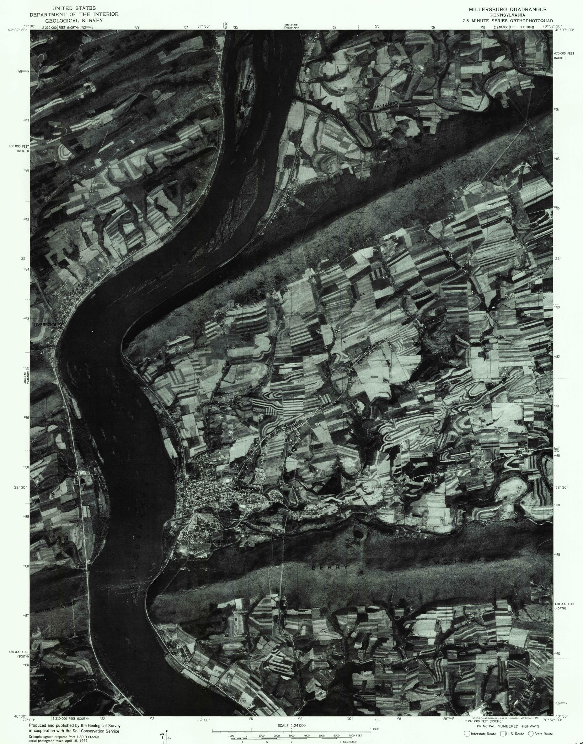
Projection: Pennsylvania coordinate system, south zone (Lambert conformal conic) 10,000-foot grid ticks based on Pennsylvania coordinate system, south and north zones 1000-meter Universal Transverse Mercator grid ticks, zone 18. 1927 North American datum Photoimagery rectified by automatic correlation
