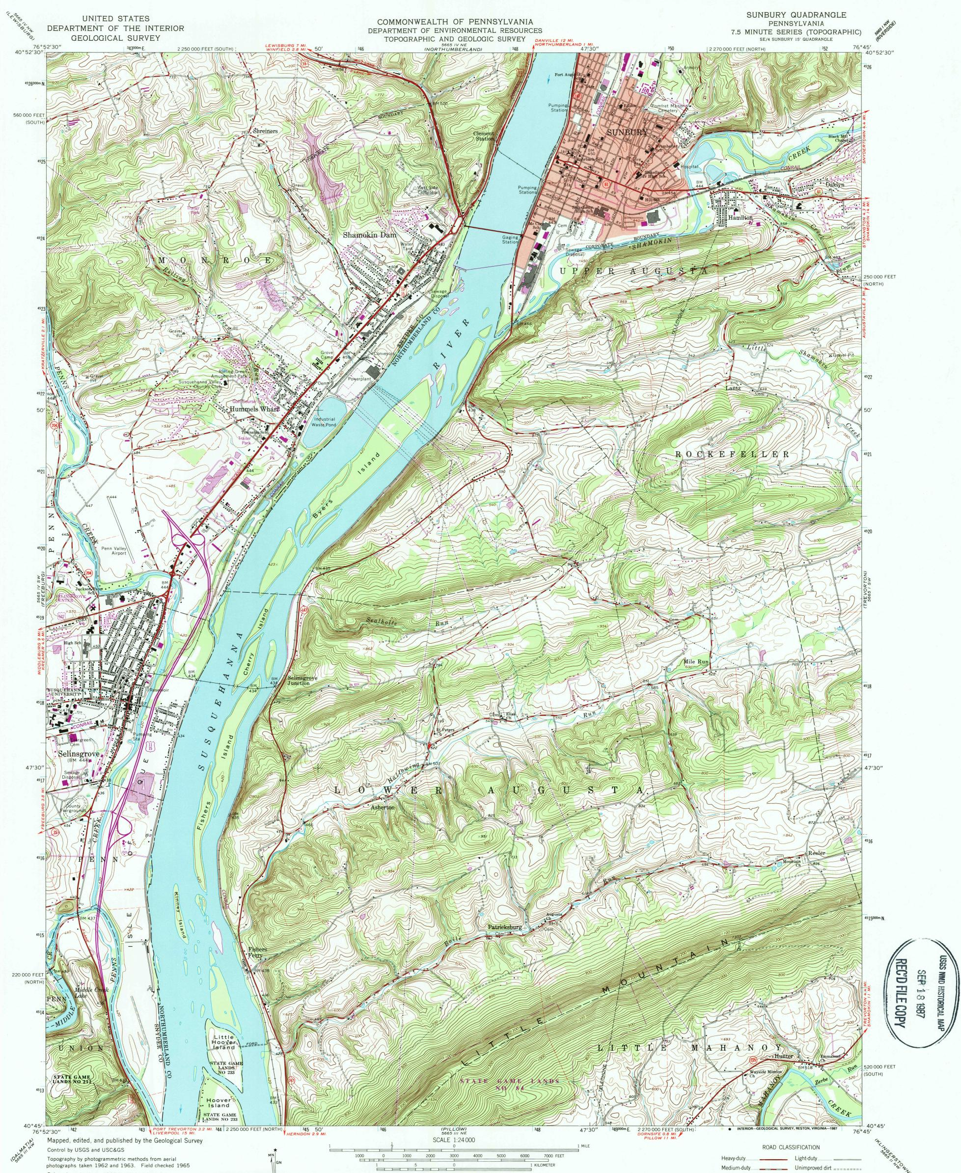
Polyconic projection. 1927 North American datum 10,000-foot grids based on Pennsylvania coordinate system, north and south zones 1000-meter Universal Transverse Mercator grid ticks, zone 18, shown in blue
