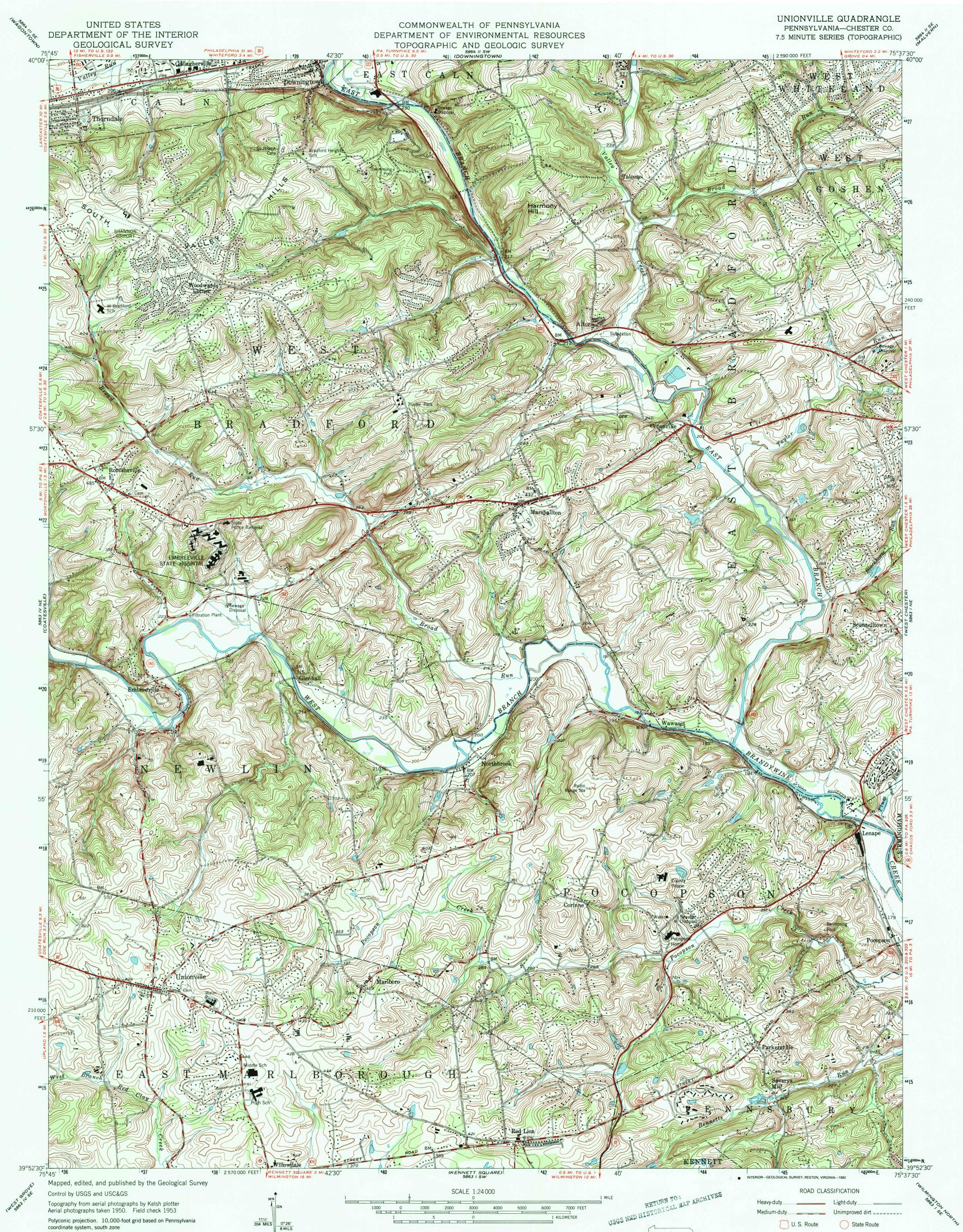
Polyconic projection. 10,000-foot grid based on Pennsylvania coordinate system, south zone 1000-meter, Universal Transverse Mercator grid ticks, zone 18; shown in blue. 1927 North American Datum The difference between 1927 North American Datum and North American Datum of 1983 (NAD 83) for 7.5-minute intersections is given in USGS Bulletin 1875. The NAD 83 is shown by dashed corner ticks
