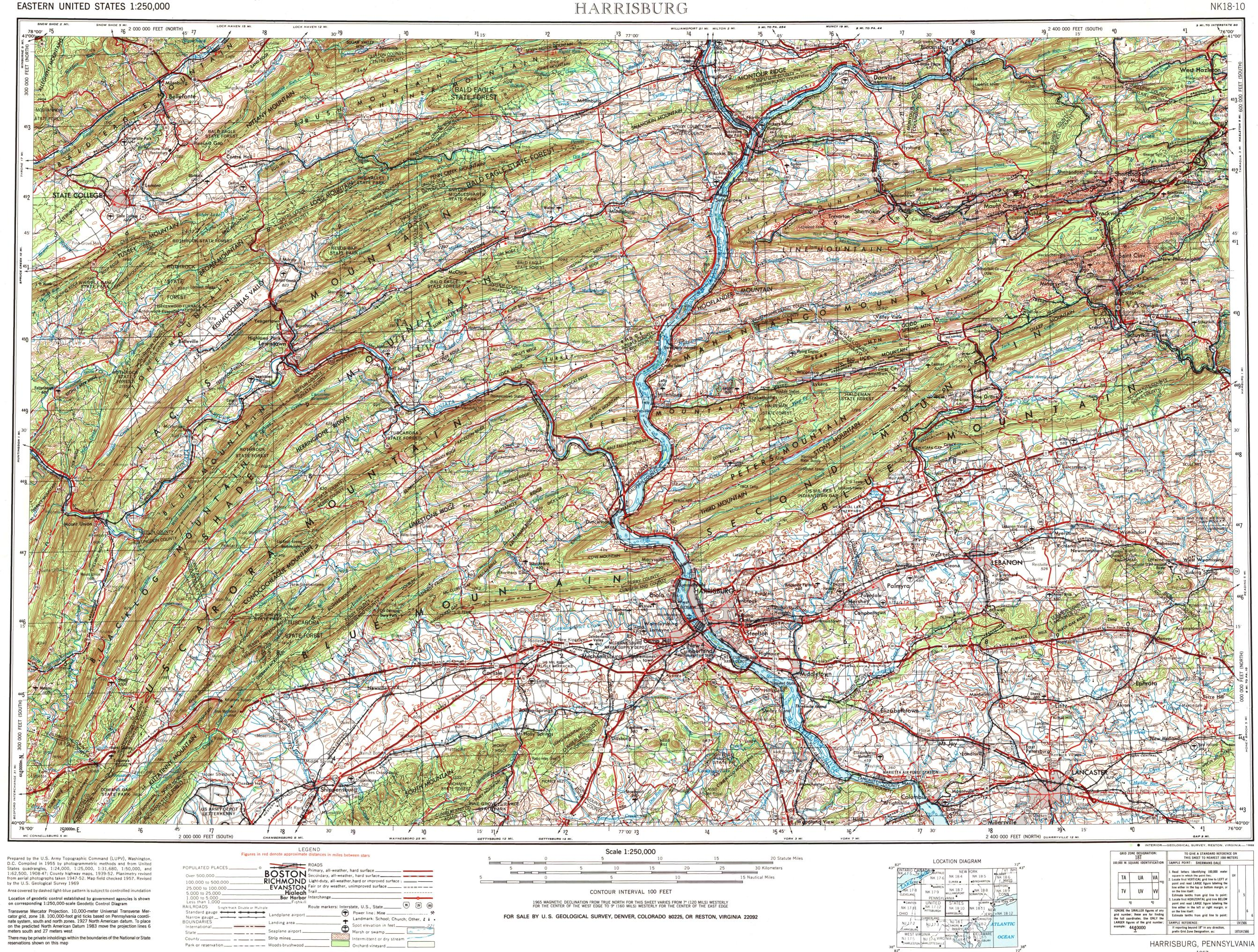
Location of geodetic control established by government agencies is shown on corresponding 1:250,000-scale Geodetic Control Diagram Transverse Mercator Projection. 10,000-meter Universal Transverse Mer-cator grid, zone 18. 100,000-foot grid ticks based on Pennsylvania coordi-nate system, south and north zones. 1927 North American datum. To place on the predicted North American Datum 1983 move the projection lines 6 meters exists and 27 meters unset meters south and 27 meters west
