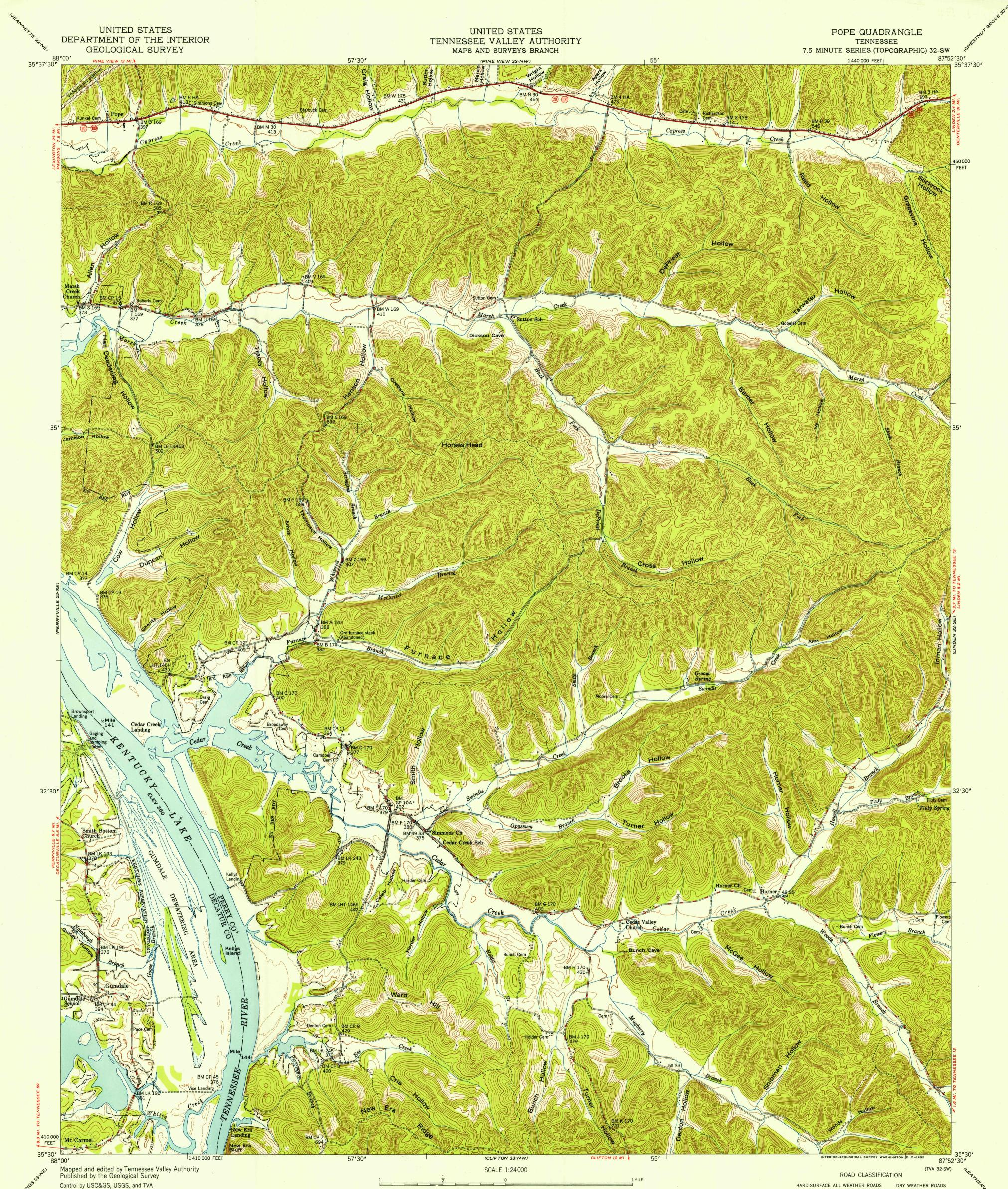
Topography by USGS and TVA by multiplex and planetable methods. Aerial photographs taken 1946 and 1952 Field examination by TVA, 1949
