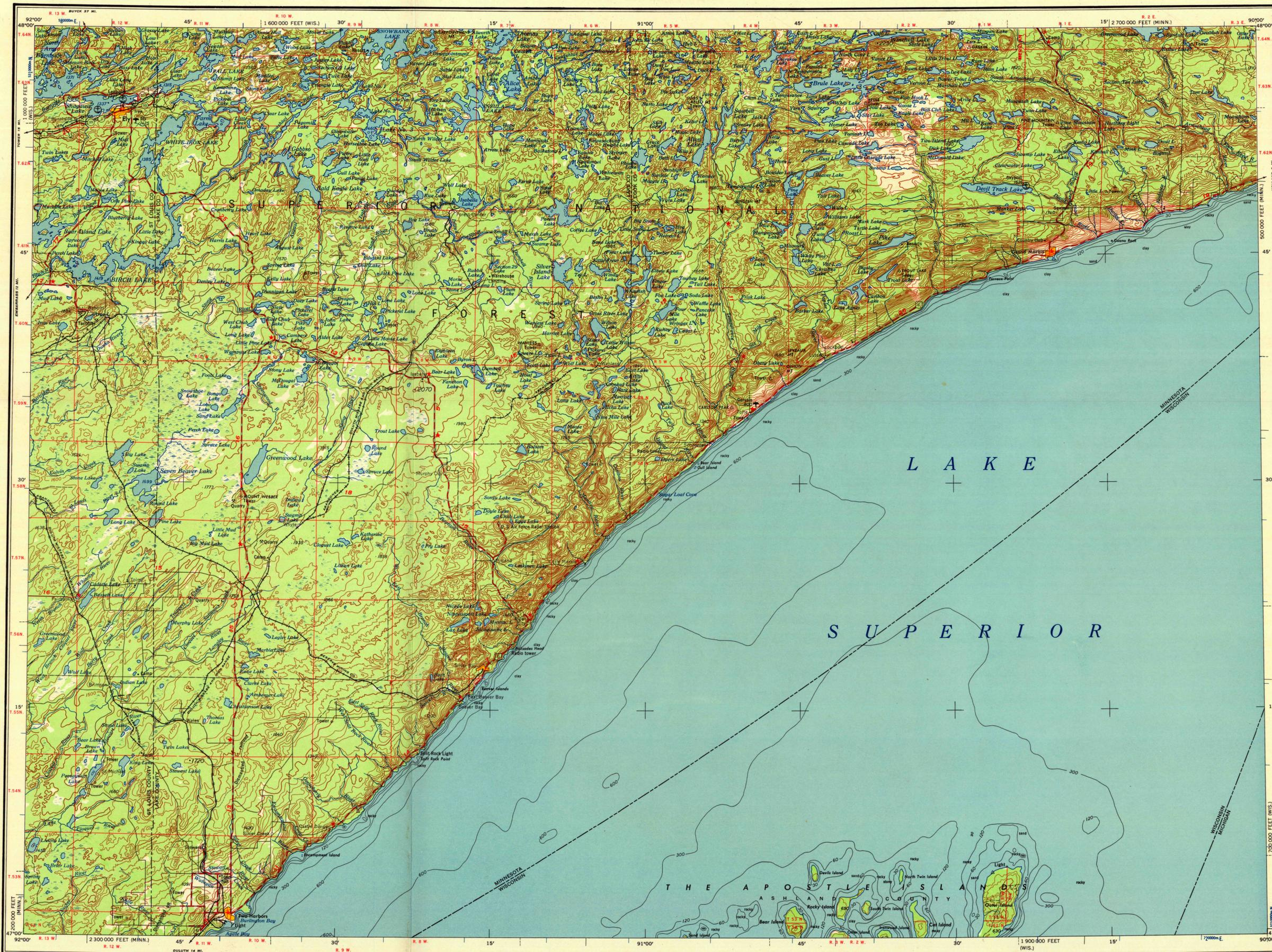
Prepared by the Army Map Service (ASGEM), Corps of Engineers, U.S. Army, Washington, D. C. Compiled in 1956 by photogrammetric methods and from: Minnesota Quadrangles, 1:24,000, USGS, 1951-1953; U.S. Lake Survey Charts 95, 96, 97, 1955. Planimetric detail revised by photogrammetric methods. Horizontal and vertical control by USGS, USFS, and USC&GS. Photography field annotated 1954.
