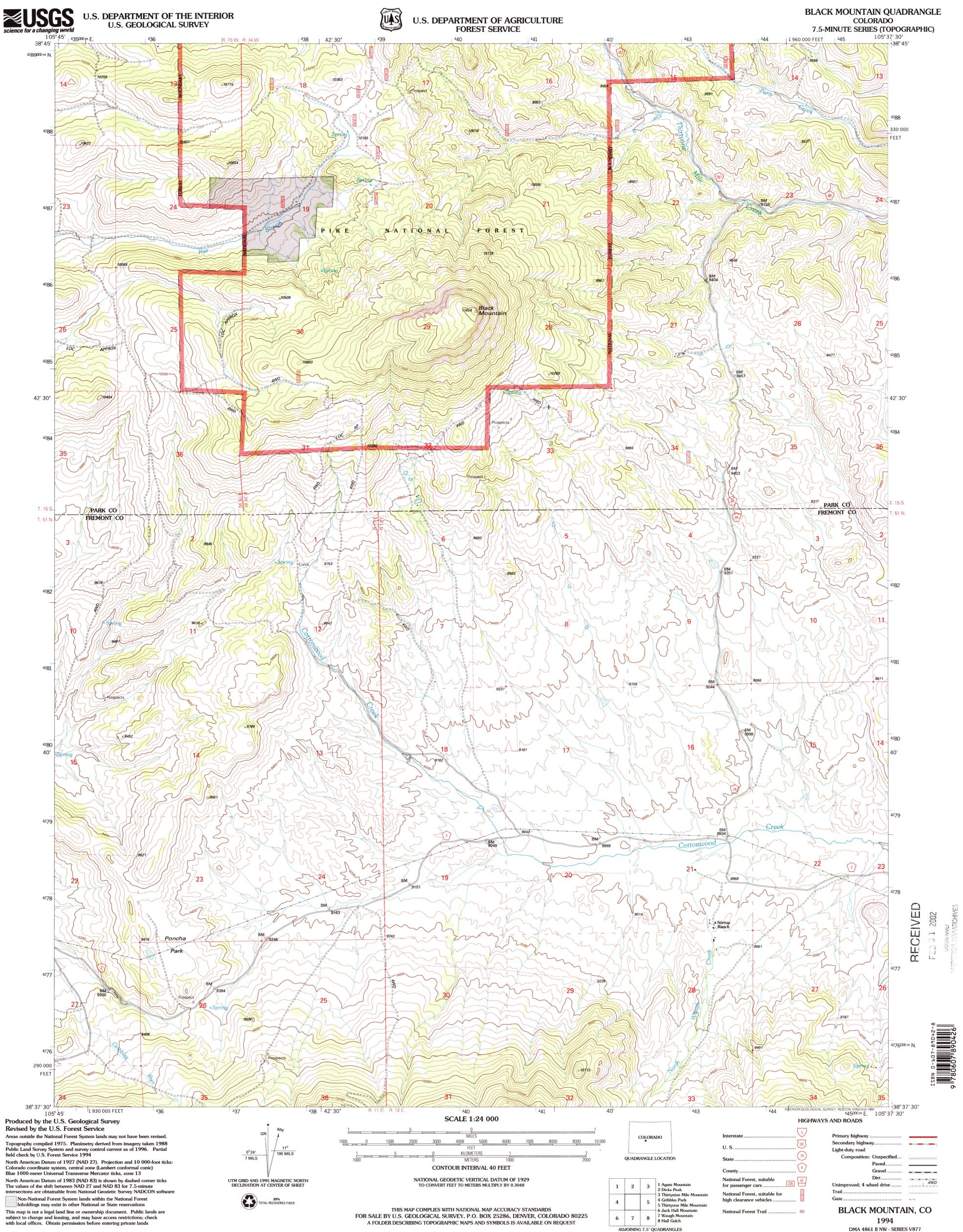
Colorado coordinate system, central zone (Lambert conformal conic) Blue 1000-meter Universal Transverse Mercator ticks, zone 13 North American Datum of 1983 (NAD 83) is shown by dashed corner ticks The values of the shift between NAD 27 and NAD 83 for 7.5-minute
